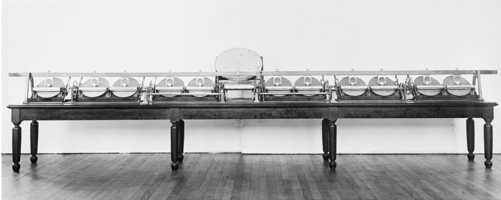
Fig. 0.7 William Thomson's first Harmonic Analyzer. 1876
