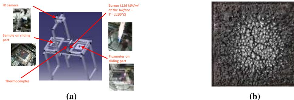
**Figure 10:** Reduced scale bench equipped with temperature rake for measuring flame temperature and with gauge for measuring heat flux impacting the sample (right); sample holder insulated from the frame (left); the two frames (right and left) are on the rail moving back and forth for calibration's purpose (a) – Intumescent coating formed after fire testing on the reduced scale ISO 2685 test (b).
