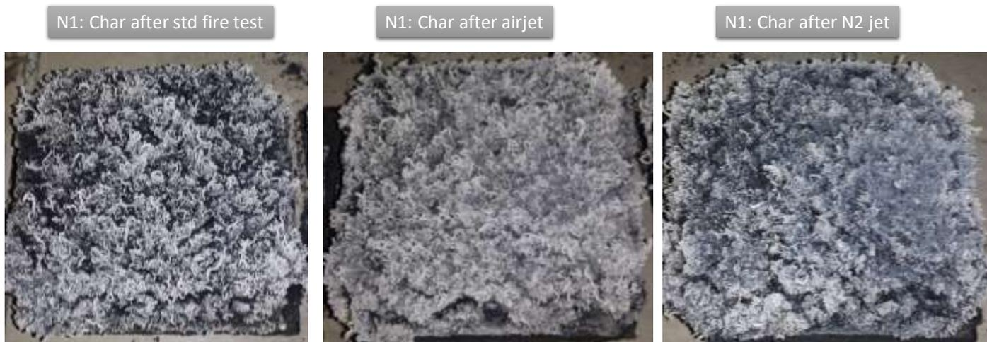
**Figure 7:** Char residues obtained in the furnace test (UL 1709) after airjet (a) and N<sub>2</sub> jet (b).
