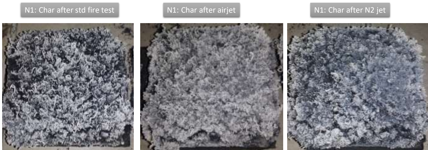
Figure 7: Char residues obtained in the furnace test (UL 1709) after airjet (a) and N 2 jet (b).
