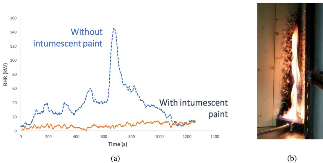
Our mini SBI was designed to be correlated with the values of the large scale SBI. It gives good prediction for the wooden panels as shown in Table 1.
