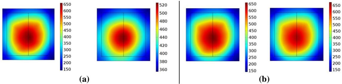
The main conclusions are temperature differences measured during the full scale ISO test compared to the virtual bench are mainly due to scaling changes. On the other hand, it was shown temperature distribution in the flame, the design of the burner and boundaries conditions had a minor influence on temperature changes.
