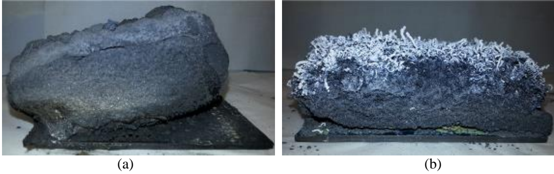
Figure 7. Intumescent char formed from intumescent coatings on steel plates, with (a) epoxy based and (b) silicon based formulations, after UL1709 hydrocarbon fire test.
