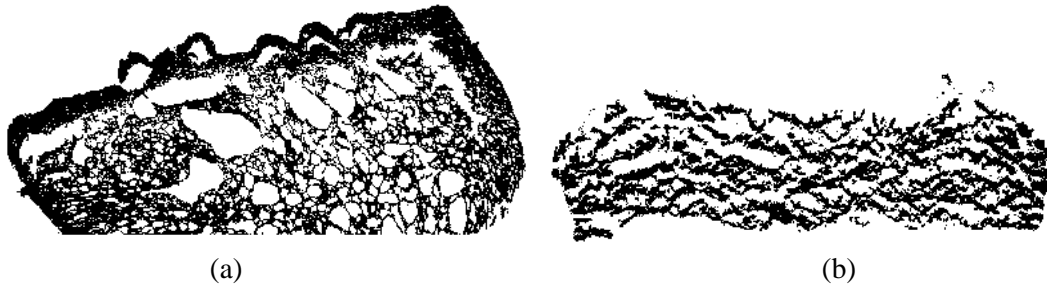
Figure 9. Binarized slice images of the inner structures of (a) epoxy based char, (b) silicon based char.
