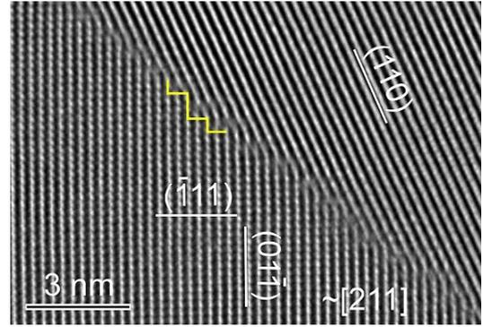
**Figure 1.1.6.** High-resolution TEM micrograph of an edge-on grain boundary in SrTiO<sub>3</sub> (Sternlicht *et al.* 2015)
