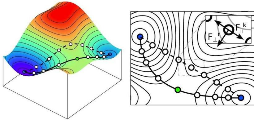
**Figure 3.1.16.** Principle of the NEB calculations. The dashed line shows the path corresponding to the initial guess for the intermediate state. After applying the NEB method, the configurations lie along the minimum energy path (solid line). The green dot on the energy landscape corresponds to the saddle point
