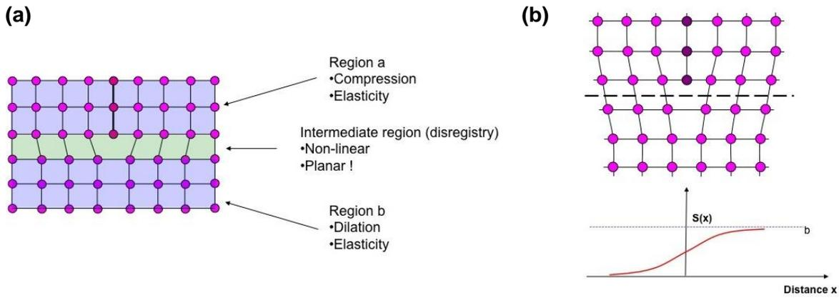
Figure 3.1.3. Schematic illustration of the PN-model principles
