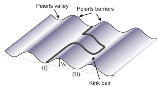
**Figure 3.1.12.** Thermal activation of dislocation glide: schematic illustration of the kink-pair mechanism which allows the dislocation line to pass from one Peierls valley to the next one at finite temperature
