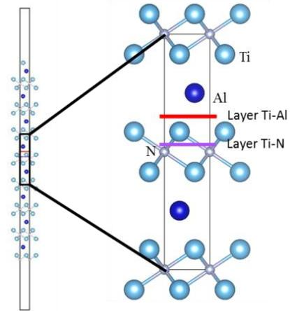
**Figure 4.5.6.** Supercell of  $Ti_2AlN$  structure used for the  $\gamma$ -surface calculations (Gouriet *et al.* 2015). The red (purple) line is the trace of (0001) between Al (N) and Ti layer. The highlighted rectangle corresponds to the unit cell
