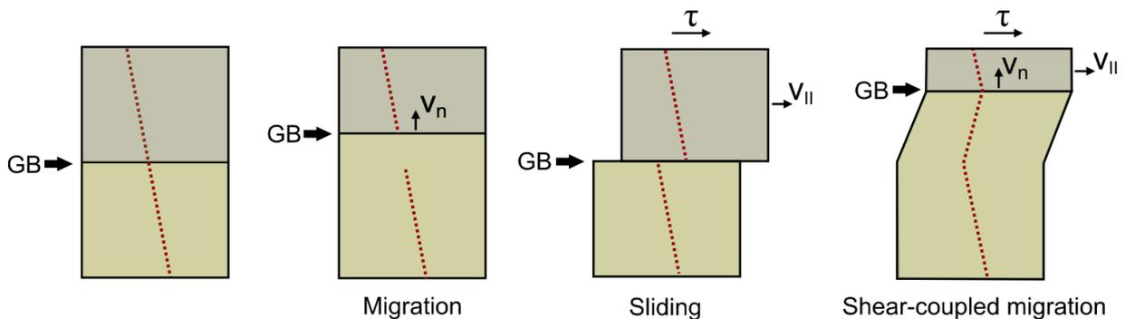
Figure 1.1.11. Different types of grain boundary motion
