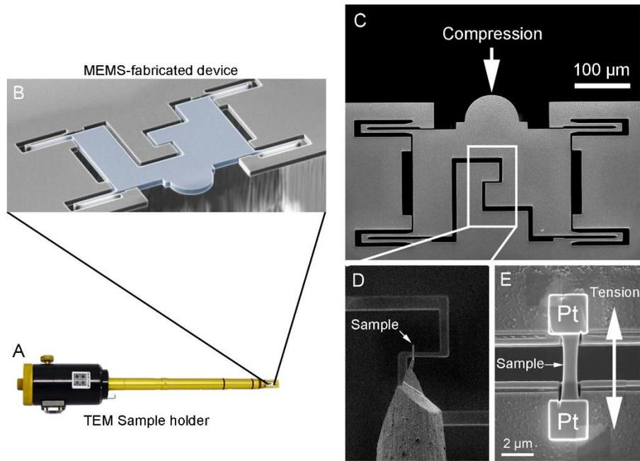
**Figure 3.3.10. Push-to-Pull (PTP) device:** (a) TEM Sample holder. (b) MEMS-fabricated PTP device. (c) Optical image of the PTP device used for in situ TEM tensile experiments. The compression of the semicircular end in (c) induces uniaxial tension in the middle gap shown in (d) and (e). (d, e) SEM images showing the transfer of an FIB-prepared olivine sample onto the PTP device and the mounting of the sample in the middle gap using electron beam-deposited platinum (Pt), respectively
