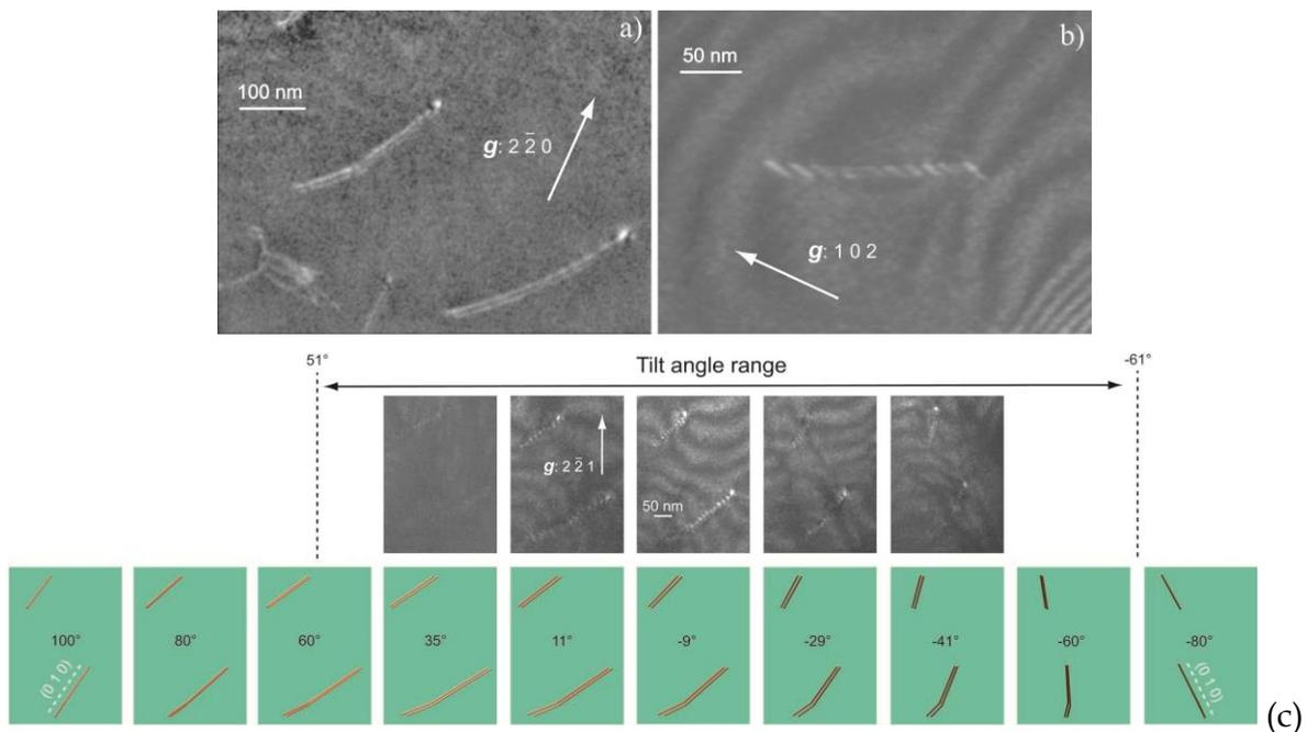
**Figure 4.5.3.** [100] dislocations in cementite. Weak-beam dark-field images show the two partial dislocations (a) and the stacking fault (b); electron tomography (c) demonstrates that [100] dislocations are dissociated in (010)
