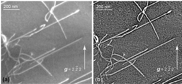
**Figure 3.3.7.** Dislocation contrast increase due to Kernel filtering and polynomial fit (Mussi *et al.* 2014)
