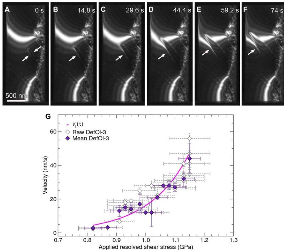
**Figure 4.1.3.** The sequence **A** to **F** illustrates successive steps of a dislocations gliding across the sample under an applied resolved shear stress of 0.89 GPa. **G** summarises the results giving the stress dependence of the velocity of [001] screw dislocations in (011)
