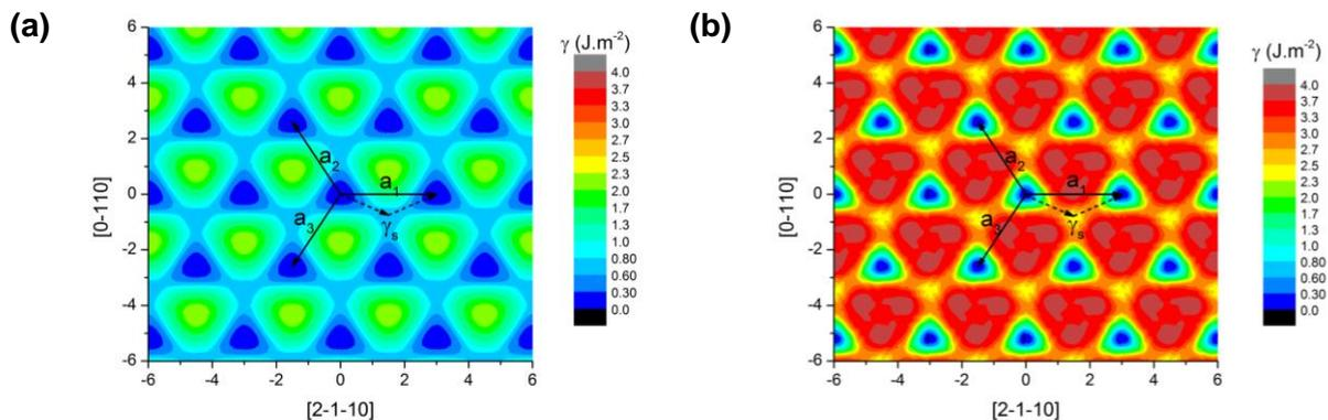
**Figure 4.5.7.**  $\gamma$ -surfaces (in  $J/m^2$ ) in (0001) with shear (a) between Ti and Al atoms and (b) between Ti and N atoms. The hexagonal base ( $a_1$ ,  $a_2$ ,  $a_3$ ) is represented,  $\gamma_s$  is the stable stacking fault with (a)  $\gamma_s = 0.72 J/m^2$  and (b)  $\gamma_s = 2.06 J/m^2$ . The dashed arrows represent the dissociation path of the dislocation with the  $a_1$  Burgers vector.
