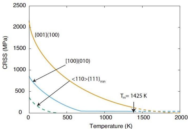
**Figure 4.5.5.** CRSS of the [100](010) and [001](100) systems in cementite as a function of temperature. Our results are compared with those of  $\langle 110 \rangle \{ 111 \}$  in ferrite from Naamane *et al.* (2010).  $T_m$  is the melting temperature of cementite
