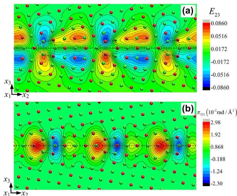
**Figure 6.1.3.** Copper: (610)/[001] tilt boundary of misorientation 18.9°. (a) In-plane Green-Lagrange shear strain  $E_{23}$ ; (b) corresponding generalized-disclination component  $\pi_{321}$
