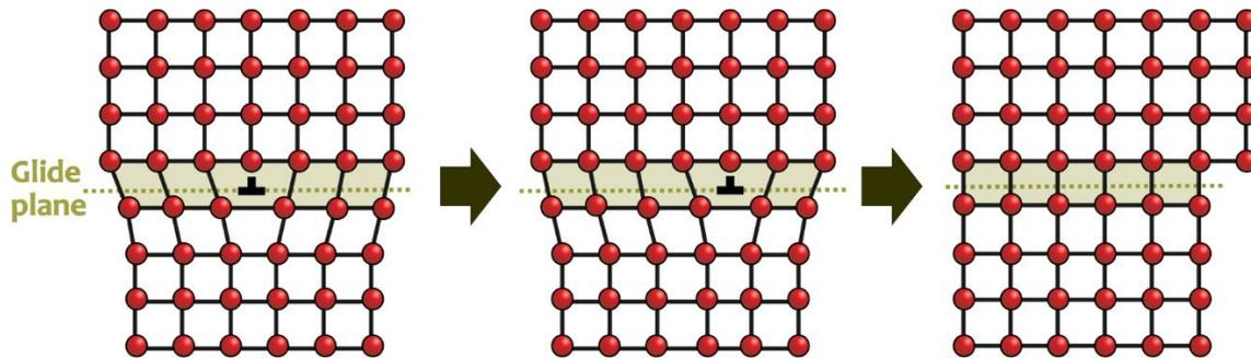
Figure 1.1.8. Schematic illustration of an edge dislocation glide
