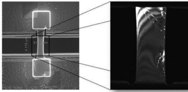
**Figure 4.1.2.** View of the experiment: a thin strip of olivine single crystal oriented for [001] slip in (011) is fixed in the push-to-pull with platinum. Right: the orientation of the foil has been chosen so as to allow good visualization of the dislocations by weak-beam dark field (see details in Idrissi *et al.* 2016)
