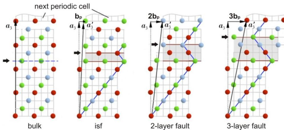
**Figure 3.1.18.** GPFE calculations at atomic scale. Location of a newly introduced shear level is indicated with a black arrow for each simulation cell. The picture is modified from the scheme provided by Kibey *et al.* (2007)
