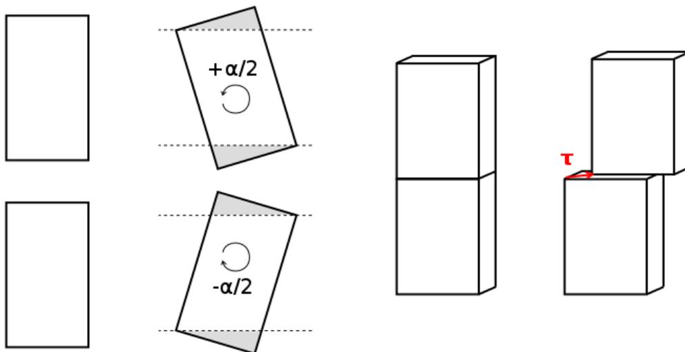
**Figure 3.1.19.** Method for the construction of symmetric tilt grain boundaries. Two single crystals are rotated by opposite angles, cut horizontally, and then stacked together. For a given misorientation  $\alpha$  between the two crystals, several relative positions along the grain boundary plane are searched, as symbolized by the translation vector  $\tau$
