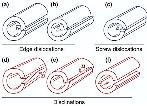
**Figure 1.1.2.** The six types of line defects introduced by Volterra (1907). The blue cylinders (a-c) illustrate translational defects, called dislocations, that are characterized by a Burgers vector  $\mathbf{b}$ ; the red cylinders (d-f) correspond to disclinations, that are characterized by a Frank vector  $\mathbf{\Omega}$  and incorporate a rotational component. The figure is adopted from Cordier et al. (2014)
