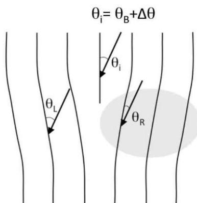
**Figure 3.3.3.** Schematic illustration depicting illumination of an edge dislocation core, slightly away from the perfect Bragg conditions. Perfect Bragg condition is only satisfied in the shaded area due to local plane bending
