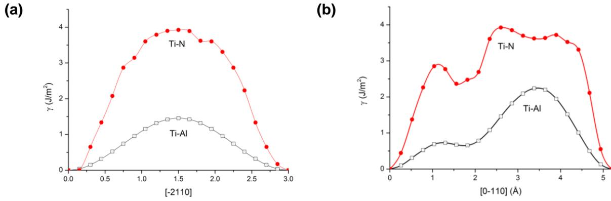
**Figure 4.5.8** (a)  $\gamma$ -line along  $[\bar{2}110]$  in (0001). (b)  $\gamma$ -line along  $[0\bar{1}10]$  in (0001). The black line and open square symbol corresponds to the (Ti-Al) layer, and the red line and circle symbol to the (Ti-N) layer
