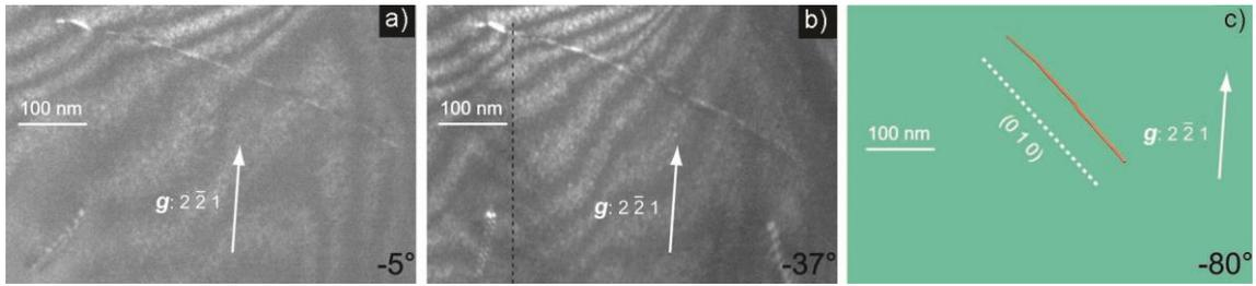
**Figure 4.5.4.** [001] dislocations in cementite. Weak-beam dark-field images show the dislocations at tilt angles  $-5^\circ$  (a),  $-37^\circ$  (b) and the reconstructed volume corresponding to a tilt angle of  $-80^\circ$  (c) which indicates the trace of the glide plane: (010)
