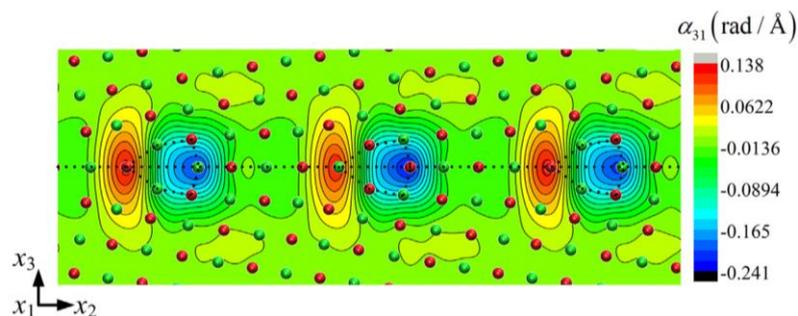
**Figure 6.1.1.** Copper: (610)/[001] tilt boundary of misorientation  $18.9^\circ$ . Edge dislocation density components  $\alpha_{31}$  on top of the relaxed atomic structure. The component  $\alpha_{31}$  renders dislocation lines of edge character aligned along the axis  $x_1$  and with their Burgers vectors along the axis  $x_3$
