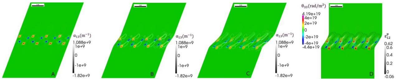
**Figure 6.1.4.** Shear-coupled boundary migration of a grain boundary made of a distribution of disclination quadrupoles. Images (A) to (C) show the downward migration of the disclinations when a positive shear strain is applied. Black and white contours show the edge dislocation density. (D) depicts the unloaded bicrystal revealing shear-coupled migration
