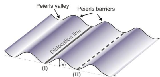
**Figure 3.1.10.** Lattice friction: schematic illustration of a straight dislocation line gliding over the Peierls potential from the valley (I) to the valley (II)
