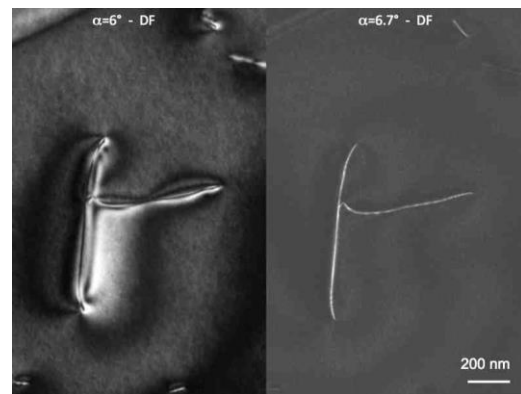
Figure 3.3.4. Change in dislocation contrast and image resolution due to a small ( 0.7^\circ ) angular deviation in dark-field imaging
