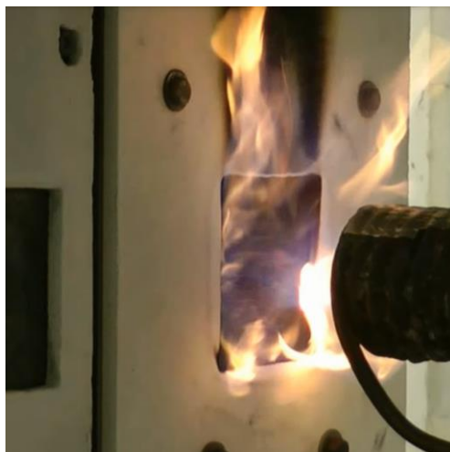
Figure 2: Picture of the burner impacting a composite material
