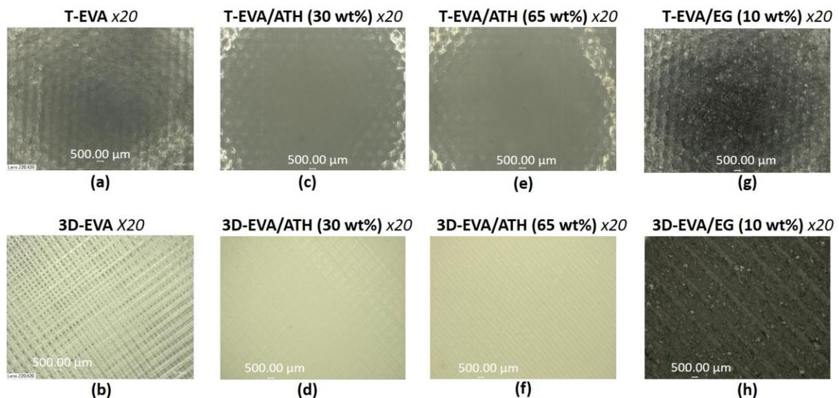
**Figure 7.** Surface observations of thermocompressed and 3D printed samples using optical microscopy x20 (a) T-EVA, b) 3D-EVA, c) T-EVA/ATH (30 wt%), d) 3D-EVA/ATH (30 wt%), e) T-EVA/ATH (65 wt%), f) 3D-EVA/ATH (65 wt%), g) T-EVA/EG (10 wt%), h) 3D-EVA/EG (10 wt%))
