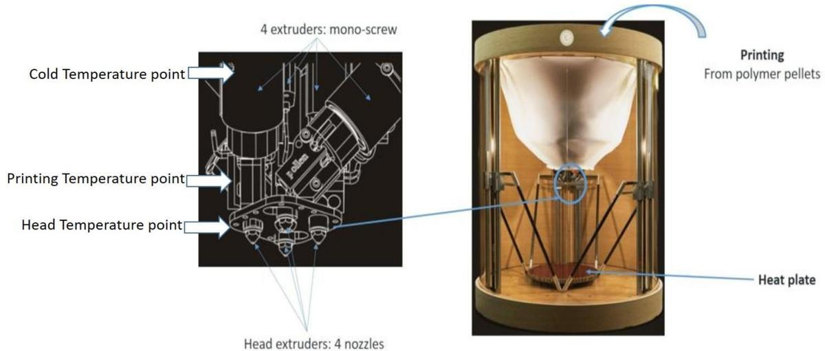
*Figure 4. Description of 3D printing used [9]*
