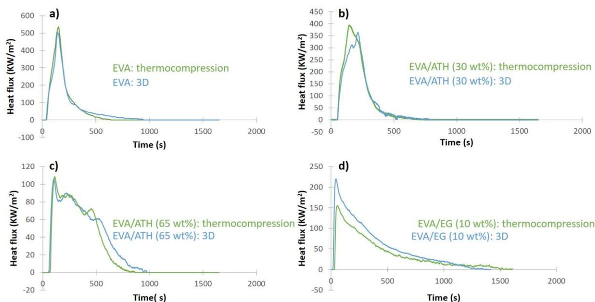
**Figure 11.** Fire behavior comparison between thermocompression and 3D printing process (a) EVA, b) EVA/ATH (30 wt%), c) EVA/ATH (65 wt%), d) EVA/EG (10 wt%)
