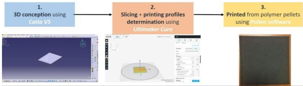
Figure 5. 3D printed process
