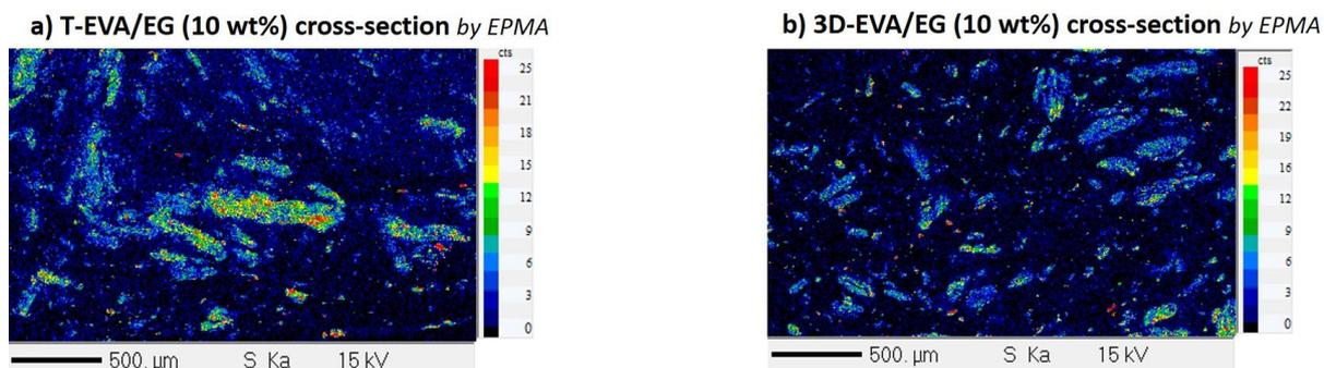
**Figure 10.** Cross-section X ray mapping in S element using EPMA measurements of (a) T-EVA/EG (10 wt%), b) 3D-EVA/EG (10 wt%)
