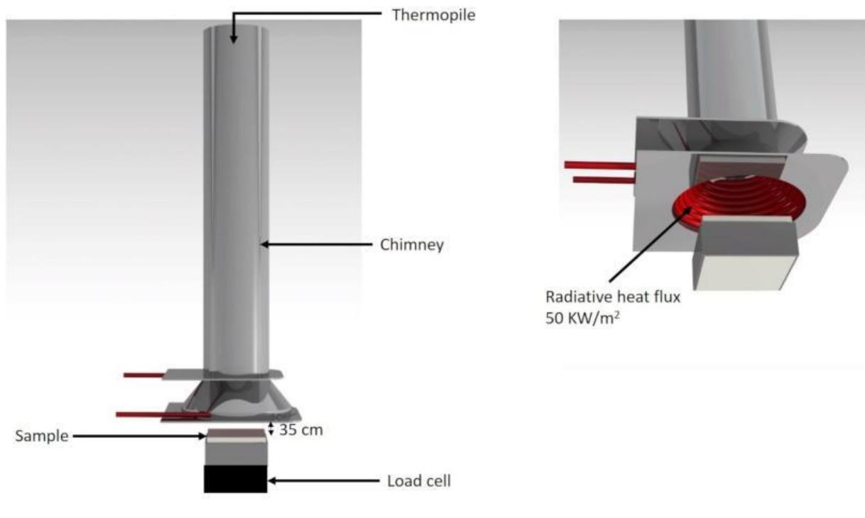
**Figure 6.** Description of Mass Loss Calorimeter (MLC) test
