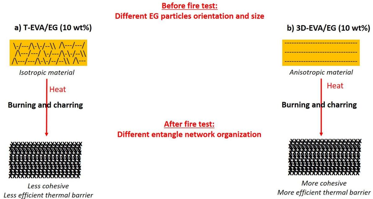
*Figure 14. Illustration of EVA/EG (10 wt%) thermal behavior (a) Thermocompressed plates, b) 3D printed plates)*
