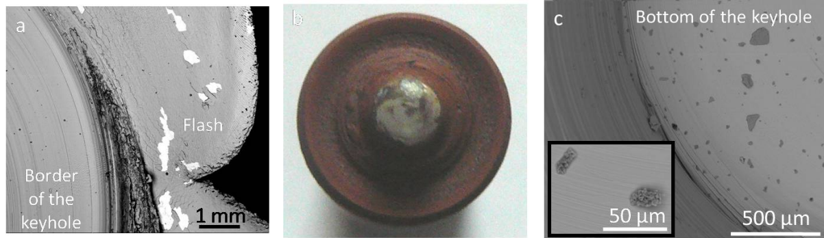
Figure 9: a) Contamination detected on the flash at the border of the keyhole of the Ni free joint (BSE/SEM). b) Tool tip after welding. c) Numerous debris at the bottom of the joint keyhole with a 0.2 mm thick Ni interlayer. The insert depicts some agglomerates of \text{Si}_3\text{N}_4 powder grains originating from the tool (BSE/SEM).
