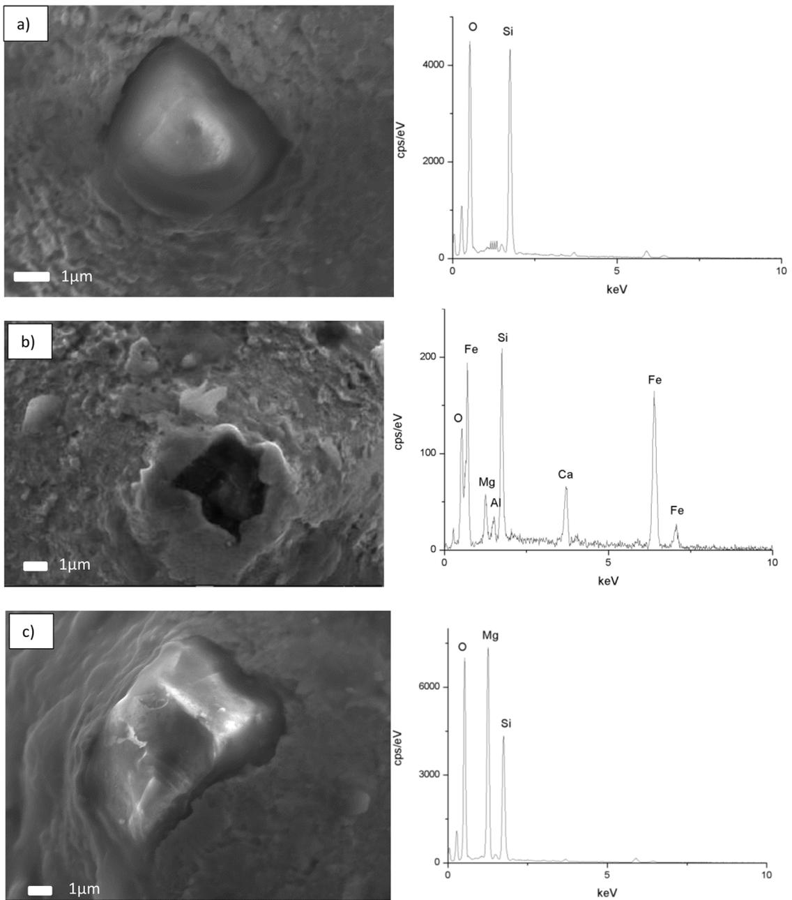
**Fig. 2.** SEM images and EDS spectra of typical inclusions found on fracture surfaces. a)  $\text{SiO}_2$ ; b)  $\text{SiO}_2\text{-CaO}$ ; c)  $\text{SiO}_2\text{-MgO}$ .
