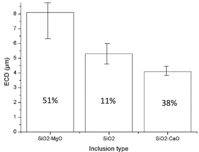
**Fig. 6.** Critical size of inclusions causing fracture.
