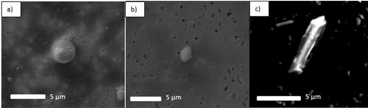
**Fig. 9.** Different inclusion morphology after dissolution. a) SiO<sub>2</sub>; b) SiO<sub>2</sub>-CaO; c) SiO<sub>2</sub>-MgO.
