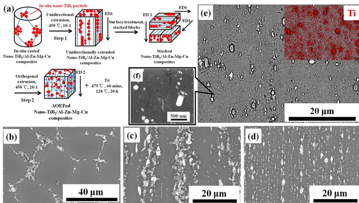
**Figure 1.** (a) The flow process chart of AOEP in this study. The SEM images of Nano-TiB<sub>2</sub>/Al-Zn-Mg-Cu composites in (b) in-situ casted state, (c) unidirectional extrusion and (d) AOEPed state, correspondingly. (e) SEM micrograph of AOEPed Nano-TiB<sub>2</sub>/Al-Zn-Mg-Cu composites after T6 treatment and the inset gives the corresponding Ti element distribution in EDX. (f) is the enlarged SEM image showing the details of nano-TiB<sub>2</sub> particles.
