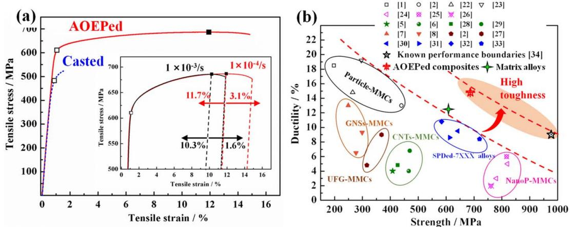
**Figure 3.** (a) The tensile strain–stress curves of the Nano-TiB<sub>2</sub>/Al-Zn-Mg-Cu composites. The hollow square is the 0.2% offset yield point and black solid square is the ultimate strength point. The inset compares the elongations of composites at a strain rate of  $10^{-3}/s$  and  $10^{-4}/s$ . (b) Strength versus tensile ductility of the AOEPed composites and matrix alloys, other Al-based MMCs and SPDED 7XXX alloys in literatures.
