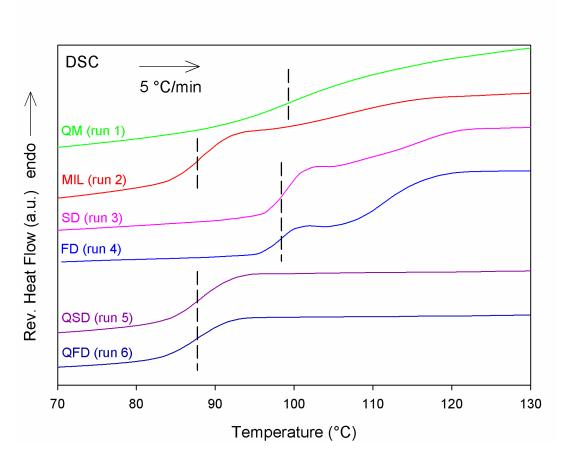
**Figure 4:** Heating MDSC curves (5 °C/min) of amorphous lactulose samples. From top to bottom: QM (green line), MIL (red line), SD (pink line), FD (blue line), QSD (purple line) and QFD (dark blue line). For reason of clarity, only the reversible signals are represented. The dashed lines mark the position of the glass transition temperature.
