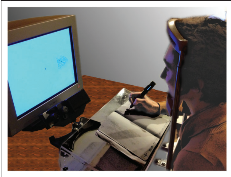
Figure 1. Experimental setup, showing (from left to right) the CRT monitor, eye tracking camera, drawing board, booklet, drawing pen, and head/chin rest.
