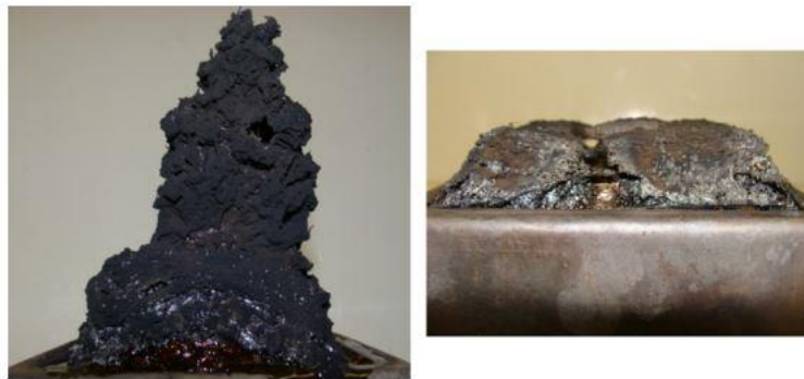
Figure 21. PC (left) and PVC (right) after exposure to a heat flux of 75kW/m 2 for 200s (initial thickness of samples was 6mm [15]).
