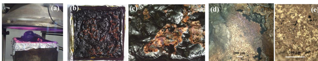
50 51 52 53 54 55 56 57 58 59 60 Figure 16. (a) Char formation as seen in MLC experiment in C2-TPU. (b) Sample collected at the onset of experiment (c) red patches on the char on the char collected at 'onset' (d,e) Focussed images on red patches.
