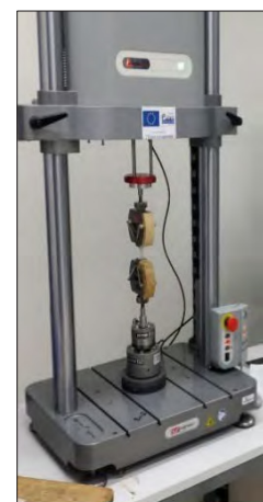
Fig. 2. Experimental setup (Instron E 3000)
