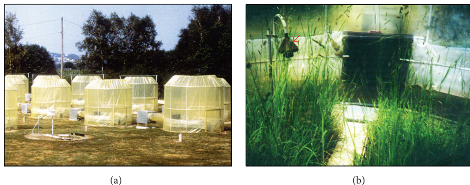
FIGURE 1: (a) Open-top chambers (OTCs) were located at Montardon site (10 km north of Pau, France). Technical characteristics of OTCs, close to those described by Heagle et al. [32, 33], have been already reported [34]. Each circular OTC had a diameter of 3 m and an open-top diameter of 2 m and was 2.8 m tall. It consisted of a galvanised iron frame covered with a polyethylene foil (Deltatex T2E). Ozone-free air (filtered air) or O_3 -enriched air was blown all around the chamber above the canopy level. The flow rate was controlled to achieve an air exchange rate of 3.14 times per min at the canopy level. When supplied, extra ozone was generated by electrical discharge of pure oxygen and injected into the air stream. Extra ozone was equally released only from 10 a.m. to 5 p.m. (GMT) in order to simulate the normal period of ozone exposure. The control chamber received filtered air (before ambient air was blown in the chamber, it passed through a charcoal filter that removed almost totally ozone), while, in O_3 -enriched OTC, O_3 concentration reached 100 \mu\text{g}/\text{m}^3 . Ozone was sequentially monitored in the three OTCs with an UV ozone analyser (Environnement SA, O_3 41 M) under the control of a computer recording system. (b) Inside a filtered air chamber: in the foreground mature Dactylis glomerata plants with inflorescences can be seen. The air suction device of the OTC allowing measurement of the ozone concentration is noted with a red arrow.
