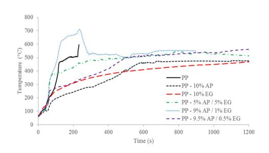
Figure 4. Temperature as a function of time at the backside of intumescent PPs during cone calorimetry experiment (external heat flux =  $35 \text{ kW.m}^{-2}$ ) – AP766 and ES 350 F5 are used as AP and EG, respectively
