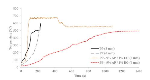
Figure 8. Temperature as a function of time at the backside of materials of different thicknesses during cone calorimetry experiment (external heat flux =  $35 \text{ kW.m}^{-2}$ ) – AP760 and ES 350 F5 are used as AP and EG, respectively
