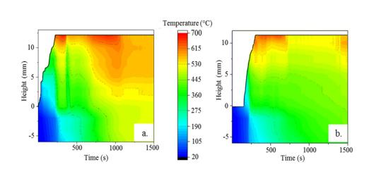
Figure 10. Mapping of temperature inside and above 6 mm thick samples of PP with AP760 / EG 350 F5 in ratios (wt% / wt%): a. 9/1; b. 10/0 during cone calorimetry experiment (external heat flux = 35 kW.m<sup>-2</sup>) – 0 mm is the height of the surface exposed to heat flux – Plain black line represents char expansion
