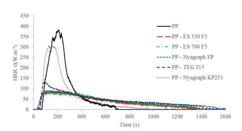
Figure 2. Heat release rate as a function of time of PP with 10wt% of different EGs during cone calorimetry experiment (external heat flux =  $35 \text{ kW.m}^{-2}$ )
