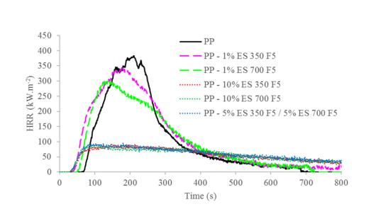
Figure 11. Heat release rate as a function of time of PP with different EGs during cone calorimetry experiment (external heat flux =  $35 \text{ kW.m}^{-2}$ )
