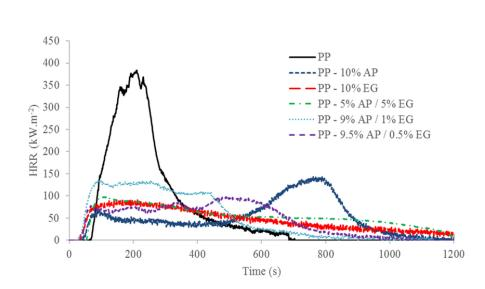
Figure 3. Heat release rate as a function of time of intumescent PPs during cone calorimetry experiment (external heat flux =  $35 \text{ kW.m}^{-2}$ ) – AP766 and ES 350 F5 are used as AP and EG, respectively
