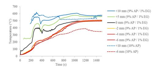
Figure 9. Temperature as a function of time inside and above 6 mm thick samples of intumescent PPs during cone calorimetry experiment (external heat flux =  $35 \text{ kW.m}^{-2}$ ) – 0 mm is the height of the surface exposed to heat flux – AP760 and ES 350 F5 are used as AP and EG, respectively
