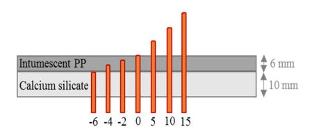
Figure 1. Arrangement of thermocouples (in orange) in 6 mm thick samples (sectional view) - Numbers are the height in mm of thermocouples compared to the surface exposed to heat flux (0 mm)
