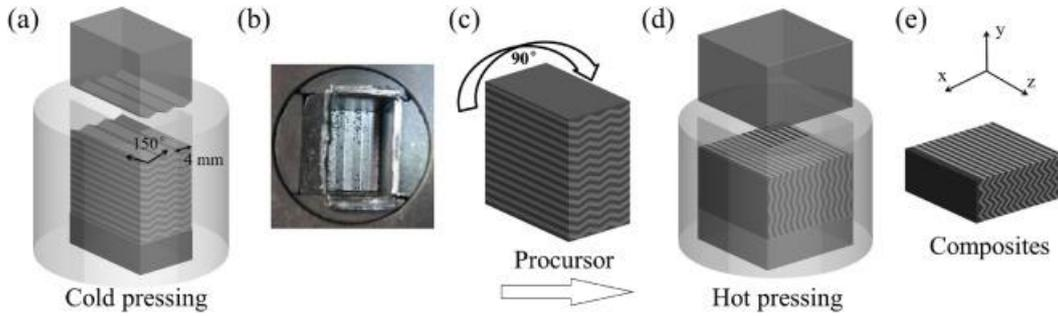
Fig. 3. Schematic illustrations of the whole fabrication process to acquire a  $G_f/\text{Al}$  composite with the 2D arrangement: (a) cold pressing using the specifically-designed punch, (b) photograph of the powder layer morphology after cold pressing, (c)  $G_f/\text{Al}$  precursor, (d) vacuum hot pressing, and (e) final product.
