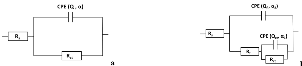
Figure 4. Equivalent circuit used to fit the impedance data for C38 steel in 1M HCl with or without XCAE according occurs (a) one phenomenon or (b) two phenomenon.
