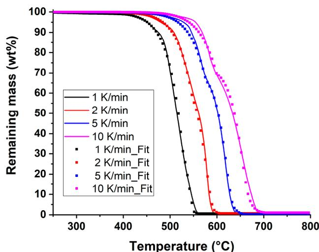
**Figure 17.** Best fit of the TG data for the three-step reaction models in Scheme 3, with the parameters given on Table 4. The curves represent the experimental data and the symbols represent the model.
