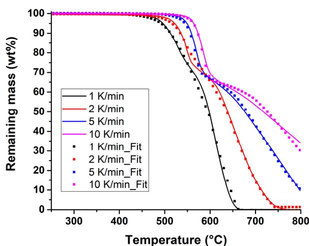
**Figure 12.** Best fit of the TG data for the three-step reaction models in Scheme 2, with the parameters given in Table 3. The curves represent the experimental data and the symbols represent the model.
