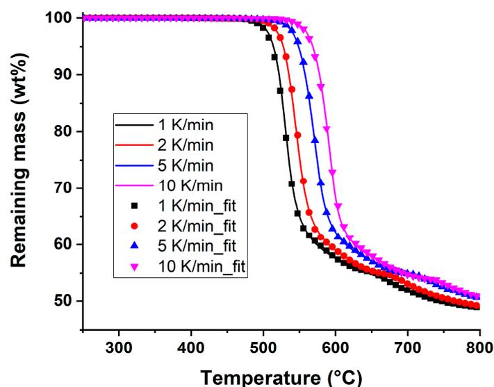
**Figure 7.** Best fit of the TG data for the three-step reaction models in Scheme 1, with the parameters given on Table 2. The curves represent the experimental data and the symbols represent the model.
