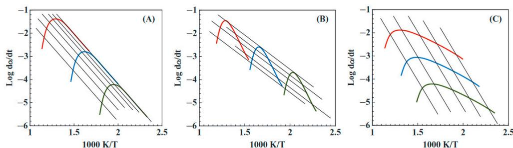
**Figure 2.** Friedman plots corresponding to a normal type of reaction (A), an accelerated reaction (B), and a retarded reaction (C). The red, blue, and green lines represent 3 different constant heating rates with red being the highest and green the lowest.
