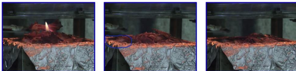
Fig. 10. Pictures taken of PI when subjected to 60 \text{ kW/m}^2 at different times during the experiment: 511 s (left), 1500 s (middle), 2400 s (right).
