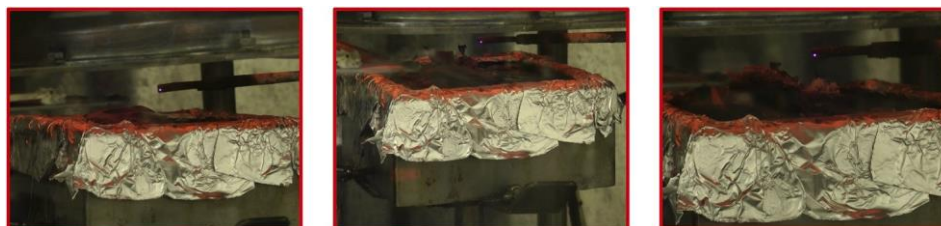
Fig. 7. Pictures taken of PI when subjected to 50 \text{ kW/m}^2 at different times during the experiment: 120 \text{ s} (left), 564 \text{ s} (middle), 1300 \text{ s} (right).
