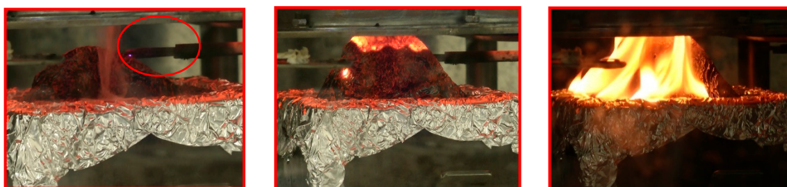
Figure 10. Pictures of PEEK taken at (left) 307 s, (middle) 852 s and (right) 889 s when it is subjected to an incident heat flux of 50 kW/m 2 using the MLC.
