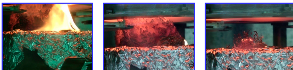
Figure 13. Photographs of PEEK under 60 \text{ kW/m}^2 at (left) 382 s, (middle) 756 s and (right) at the end of the test.
