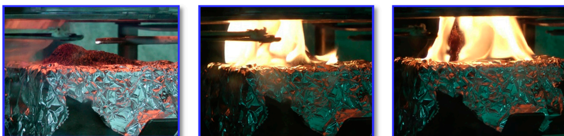
Figure 12. Photographs of PEEK when subjected to 60 \text{ kW/m}^2 under the MLC at different times. (left) 79 s; (middle) 150 s; (right) 252 s.
