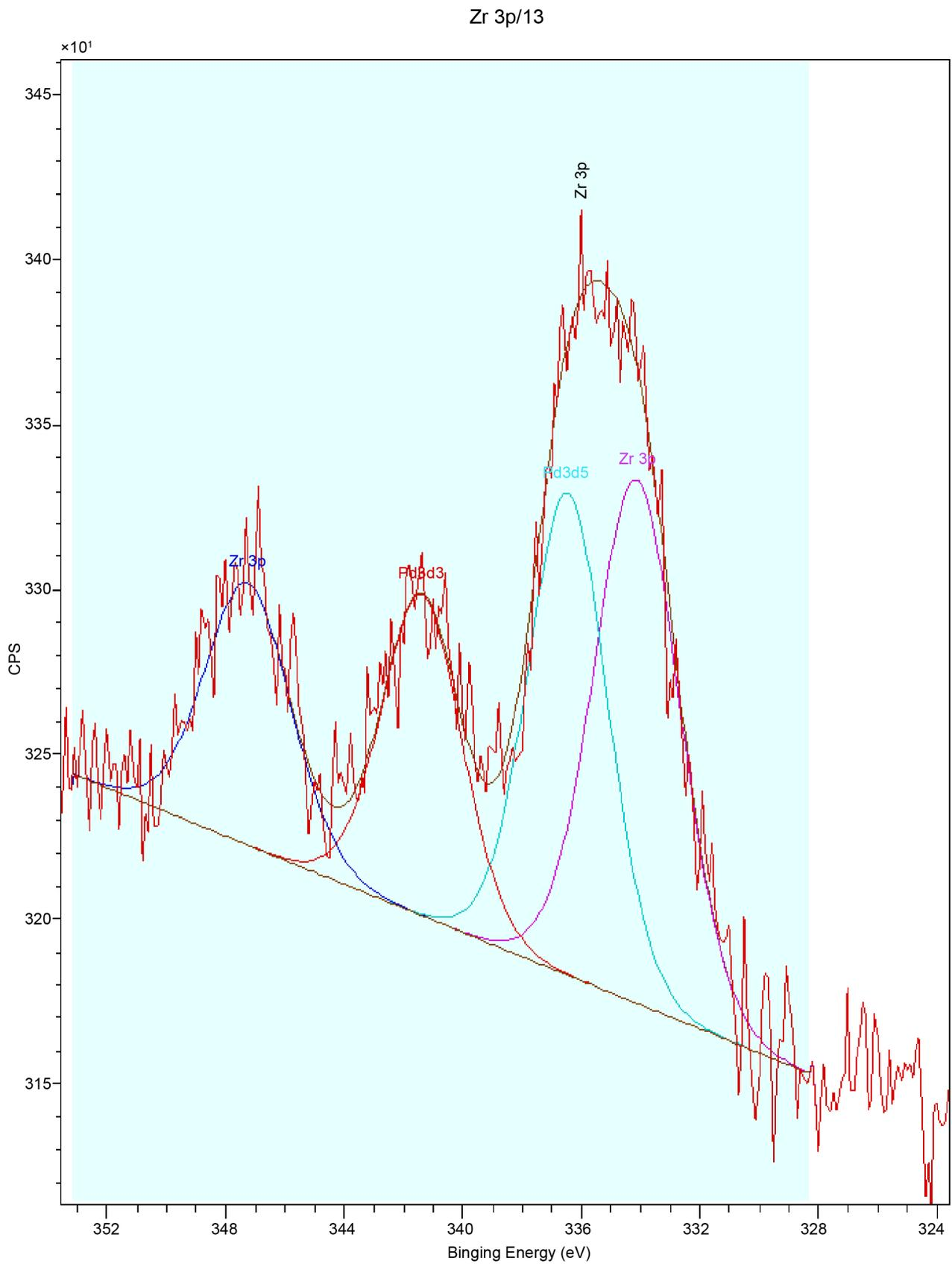
**Figure 3.** XPS patterns of the Pd/(Ce<sub>0.33</sub>Zr<sub>0.66</sub>O<sub>2</sub>)SiO<sub>2</sub> catalysts: (a) CeZr2, (b) CeZr4 and (c) CeZr8.
