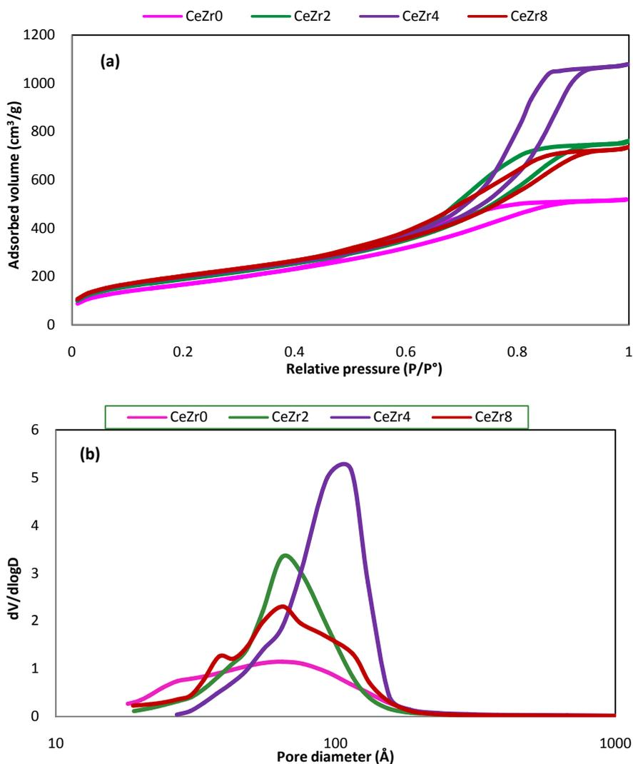
**Figure 1.** (a) Effect of the Zr and Ce loadings on the adsorption-desorption isotherm profile of the Pd/(Ce<sub>0.33</sub>Zr<sub>0.66</sub>O<sub>2</sub>)SiO<sub>2</sub> samples. (b) Average pore diameter distributions of the Pd/(Ce<sub>0.33</sub>Zr<sub>0.66</sub>O<sub>2</sub>)SiO<sub>2</sub> samples.
