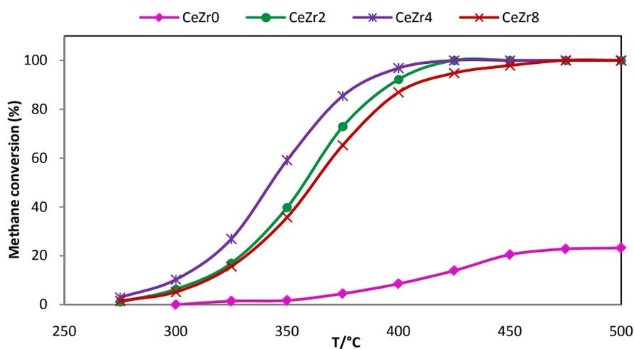
**Figure 5.** Effect of the Zr and Ce loadings on the activity of Pd/(Zr<sub>0.66</sub>Ce<sub>0.33</sub>O<sub>2</sub>)SiO<sub>2</sub> catalysts.**Table 4.** Light-off temperature and turnover number at 325 °C of the Pd/(Ce<sub>0.33</sub>Zr<sub>0.66</sub>O<sub>2</sub>)SiO<sub>2</sub> catalysts.
