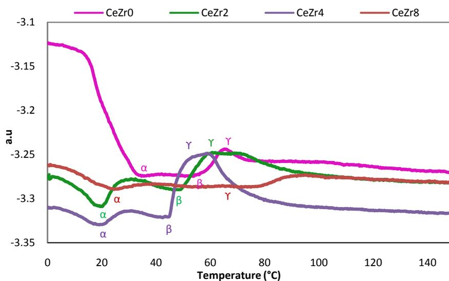
**Figure 4.** TPR profiles of the Pd/(Ce<sub>0.33</sub>Zr<sub>0.66</sub>O<sub>2</sub>)SiO<sub>2</sub> catalysts.
