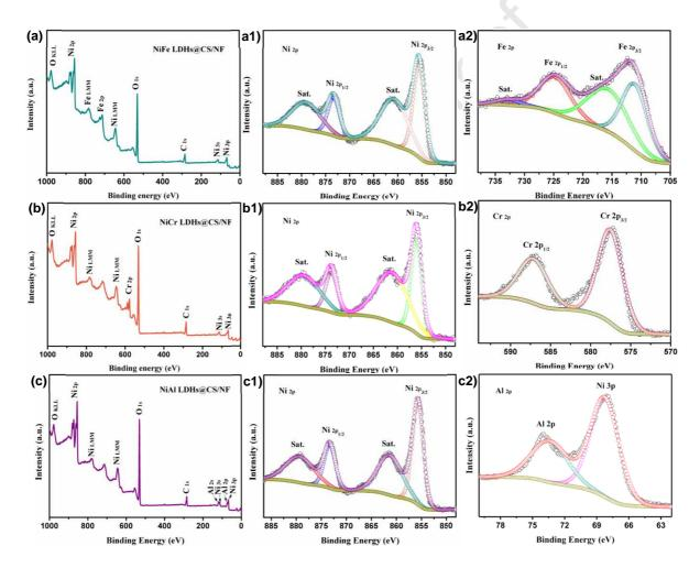
Figure 6: XPS analysis: (a) Survey and core level spectra of (a1) Ni<sub>2p</sub> and (a2) Fe<sub>2p</sub> of NiFe LDHs@CS/NF. (b) Survey and core level spectra of (b1) Ni<sub>2p</sub> and (b2) Cr<sub>2p</sub> of NiCr LDHs@CS/NF. (c) Survey and core level spectra of (c1) Ni<sub>2p</sub> and (c2) Al<sub>2p</sub> of NiAl LDHs@CS/NF.
