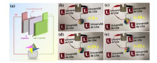
**Figure 11.** (a) Schematic diagram of the hybrid supercapacitor device for operating a homemade windmill device. (b-e) Photographs of the home-designed windmill device operation.
