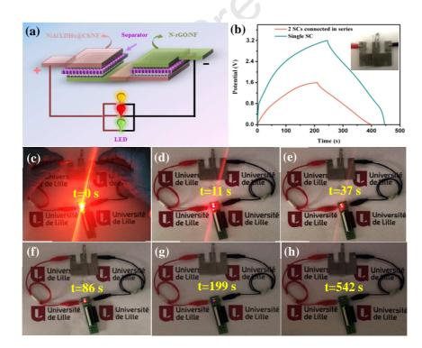
**Figure 12.** (a) Schematic diagram of the hybrid supercapacitor in series for lighting of LEDs in parallel. (b) GCD plots of a single supercapacitor and two supercapacitors in series. The inset depicts the photograph of the two supercapacitors devices in series. (c to h) A yellow LED, a red LED and a green LED in parallel lighted up by two supercapacitors in series.
