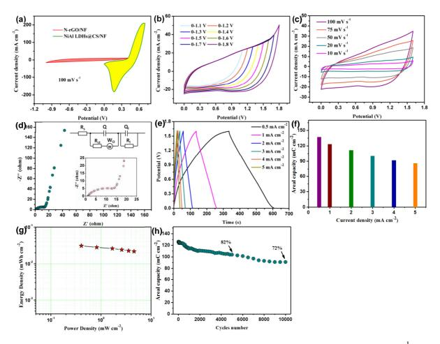
Figure 8: (a) CV curves of N-rGO/NF and NiAl LDHs@CS/NF performed at 100 mV s<sup>-1</sup> in a 3-electrode cell in KOH (2M) solution. (b) CV plots of the hybrid supercapacitor cell acquired at various potential windows (scan rate=100 mV s<sup>-1</sup>) in a classical 2-electrode configuration. (c) CV plots of the hybrid supercapacitor cell obtained at various scan rates. (d)
