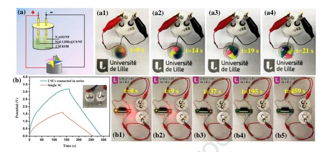
**Figure 9.** (a) Schematic of the hybrid supercapacitor cell operating a homemade windmill device. (a1 to a4) Photographs of the home-designed windmill device operation. (b) GCD curves of a single supercapacitor and two supercapacitors in series. The inset depicts the photograph of the two supercapacitors in series. (b1 to b5) A red LED, a green LED and a yellow LED in parallel lighten up by two supercapacitor cells in series.
