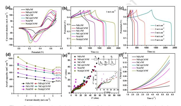
Figure 7: The electrochemical characteristics of the electrodes measured in a classical
