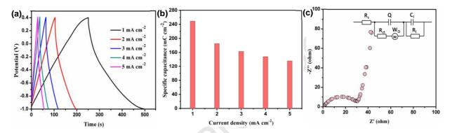
**Figure 3:** The electrochemical behavior of N-rGO in 2 M KOH solution. (a) GCD plots at various current densities. (b) Areal capacity values at various current densities. (c) EIS acquired at open circuit potential in the frequency range of 0.01 Hz to 100 kHz.
