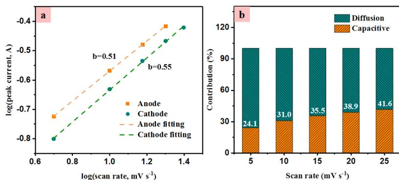
**Figure 5:** (a) Relationship between  $\log(i)$  and  $\log(v)$  of  $\text{Ni}(\text{OH})_2@\text{CuO}@\text{Cu}-150$ . (b) Capacitive contribution ratio of  $\text{Ni}(\text{OH})_2@\text{CuO}@\text{Cu}-150$  at various scan rates.
