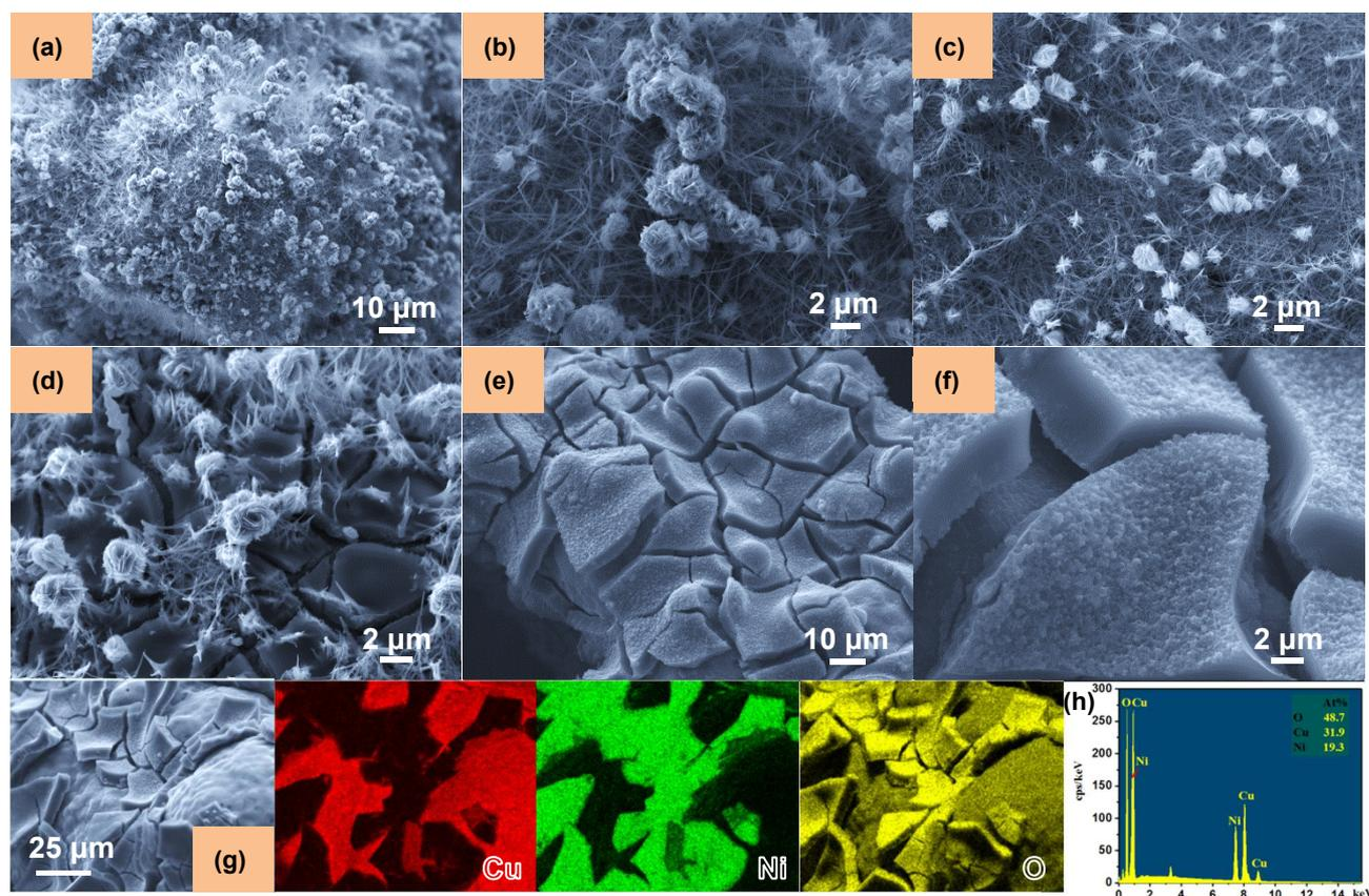
**Figure 2:** SEM images of (a,b) CuO@Cu foam, (c) Ni(OH)<sub>2</sub>@CuO@Cu-30, (d) Ni(OH)<sub>2</sub>@CuO@Cu-90 and (e,f) Ni(OH)<sub>2</sub>@CuO@Cu-150. (g) EDS elemental mapping images and EDS spectrum of Ni(OH)<sub>2</sub>@CuO@Cu-150.
