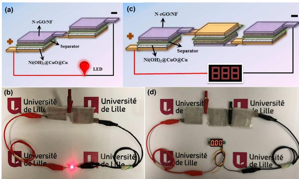
**Figure 7.** (a) Schematic diagram of two hybrid supercapacitor devices in series for lighting of a LED. (b) A red LED lighted up by two supercapacitor devices in series. (c) Schematic diagram of three hybrid supercapacitor devices in series for lighting a digital display. (d) A three-digit digital display lighted up by three supercapacitor devices in series.
