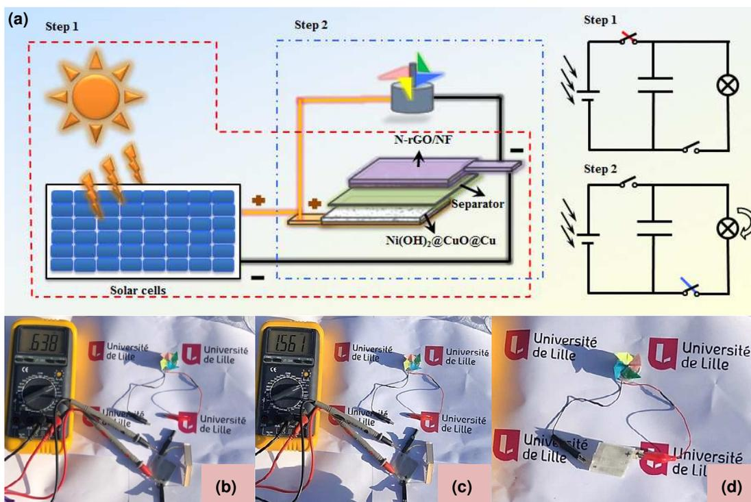
**Figure 8.** Schematic diagram and equivalent circuit of integrated system combining solar cells with the hybrid supercapacitor device for operating a homemade windmill device. (b-c) Photographs of the solar cells charging of the hybrid supercapacitor device. (d) Photograph of the home-designed windmill device operation.
