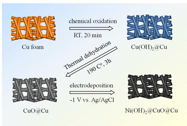
**Figure 1:** Illustration of the synthesis of Ni(OH)<sub>2</sub>@CuO@Cu electrode.
