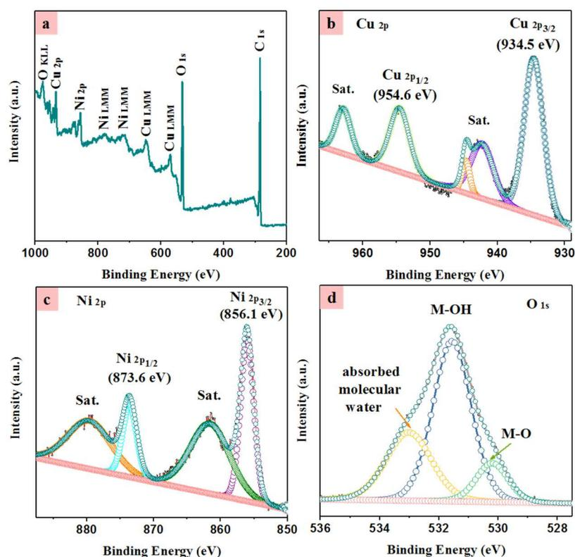
**Figure 3:** XPS analysis of  $\text{Ni(OH)}_2\text{@CuO@Cu-150}$ : (a) Survey spectrum, and core-level spectra of (b)  $\text{Cu}_{2p}$ , (c)  $\text{Ni}_{2p}$  and (d)  $\text{O}_{1s}$ .
