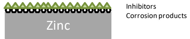
Fig. 7. Bode phase diagram for zinc in 3% NaCl and schematic describing the evolution of the covering of the zinc surface versus EEBGP concentration in 3% NaCl: (a) without inhibitor, (b) with addition of EEBGP and (c) with addition of optimum concentration of EEBGP .
