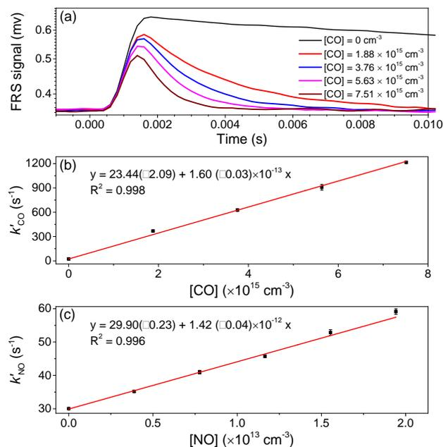
**Figure 6.** (a) Examples of the measured OH decay FRS signals of zero air and different concentrations of CO, and a plot of the pseudo-first-order decay rates versus reactant concentration: (b) CO and (c) NO. The laser frequency was fixed at the peak position of the OH absorption.
