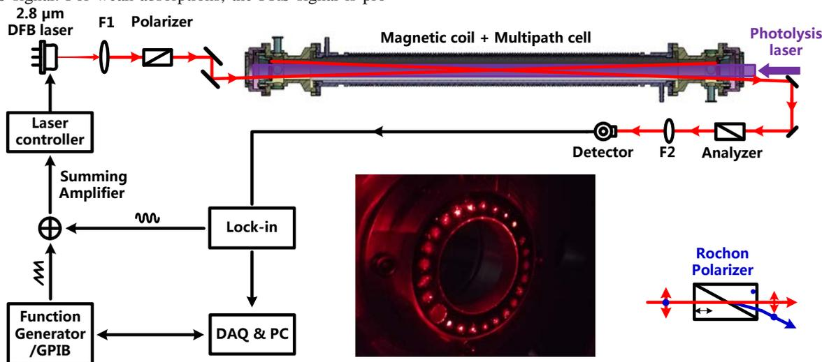
**Figure 1.** A schematic of the LFP-FRS system and a photograph of the light spot pattern in the Herriott-type multipass cell. Both the polarizer and the analyzer used were Rochon type prisms. F: lens, DAQ: data acquisition, PC: personal computer.
