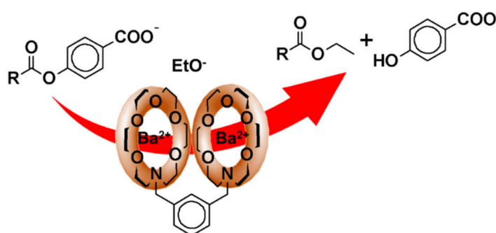
Figure 12. Transesterification by a dinuclear barium complex.
