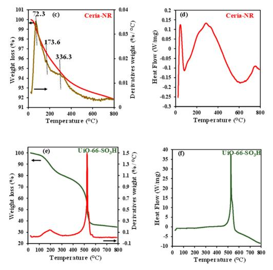
**Figure 4.** Weight loss  $(\mathbf{a}, \mathbf{c}, \mathbf{d})$  and heat flow  $(\mathbf{b}, \mathbf{e}, \mathbf{f})$  profiles during TGA-DTG analysis of Hopcalite  $(\mathbf{a}, \mathbf{b})$ , CeO<sub>2</sub>-NR  $(\mathbf{c}, \mathbf{d})$  and UiO-66-SO<sub>3</sub>H  $(\mathbf{e}, \mathbf{f})$ .
