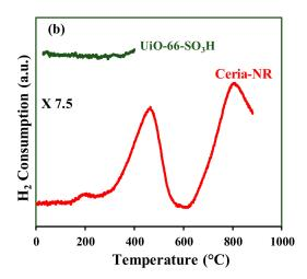
**Figure 3.** (a) H<sub>2</sub>-TPR curves of the samples; (b) zoom of the H<sub>2</sub>-TPR curves.
