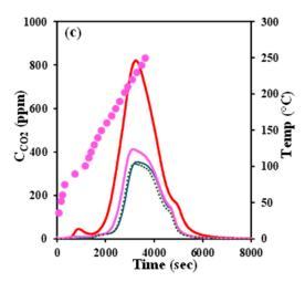
**Figure 6.** (a) Breakthrough curves of Hopcalite at different initial toluene concentration (dotted line corresponds to the concentration of toluene) (b) TPD profile of toluene (c) TPR profile of CO<sub>2</sub> (circle represent the temperature).
