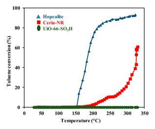
**Figure 5.** Light-off curves obtained in the presence of Hopcalite, Ceria-NR and UiO-66-SO<sub>3</sub>H for toluene oxidation.
