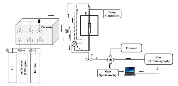
**Figure 8.** Schematic diagram of the experimental set-up used for abatement of toluene by adsorption/catalytic oxidation.
