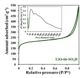
Figure 2.  $N_2$  adsorption/desorption isotherms and PSD (inserts) of Hopcalite, Ceria-NR and UiO-66-SO<sub>3</sub>H.
