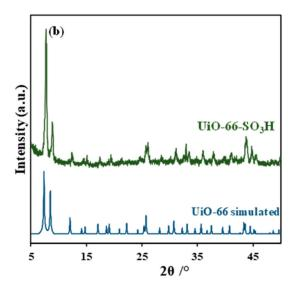
Figure 1. XRD patterns of (a): Hopcalite and CeO<sub>2</sub>-NR, (b): UiO-66-SO<sub>3</sub>H.
