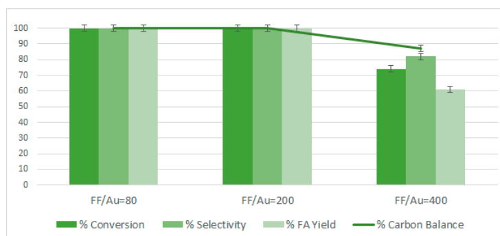
Figure 9. Effect of the FF/Au molar ratios using Au/HT 4:1 catalyst. Furfural oxidation, batch reactor, p = 6 bar ( O_2 ), t = 110 °C, 600 rpm, 2h, [FF] = 26 mM.
