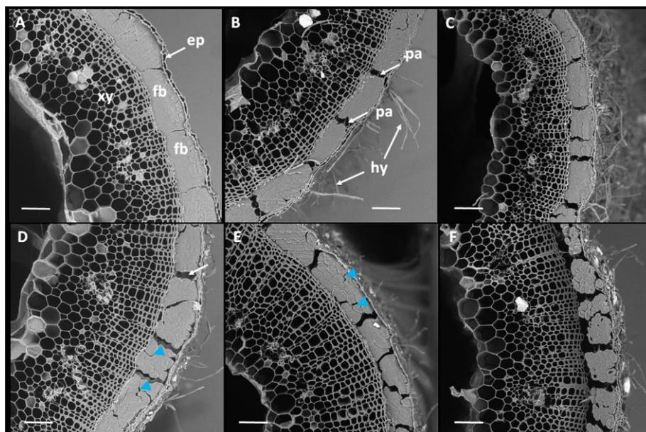
**Figure 3:** SEM imaging of transverse sections of flax stem at different retting stages: A) R0, B) R2, C) R4, D) R6, E) R7, F) R8; xy, xylem; fb, fiber bundles; pa, parenchyma, ep, epidermis; hy, hypha. White arrows and blue arrowheads indicate inter- and intra-bundle dissociation respectively. Scale bar = 100  $\mu$ m
