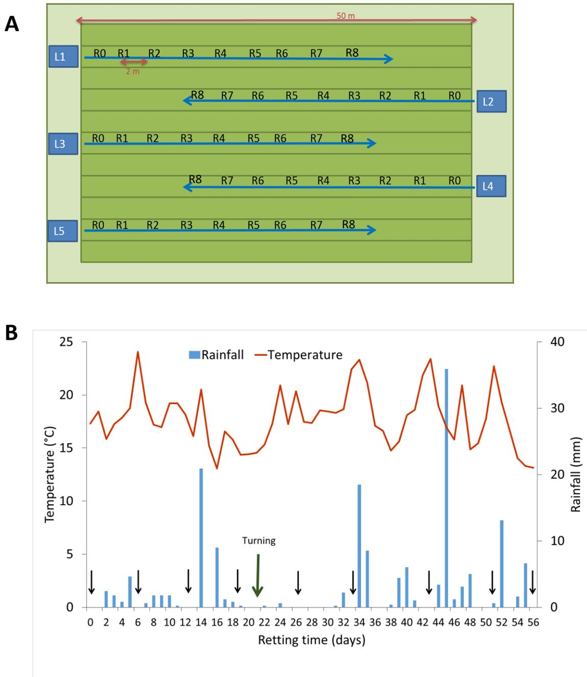
**Figure S1** : Experimental conditions of field retting: A) experimental plots B) climatic conditions. Samplings are labeled as R0 to R8 on each of the 5 replicates at regular intervals (see B, black arrows). The swath were turned once during retting (see B, green arrow)
