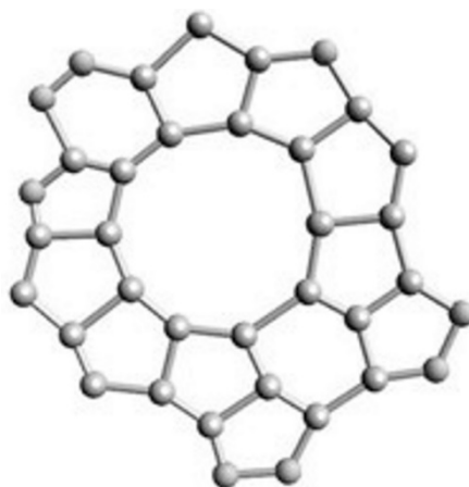
Figure 10. Schematic drawing of synthetic ZSM-5 zeolite. Reprinted from Reference [84], with permission from Elsevier.
