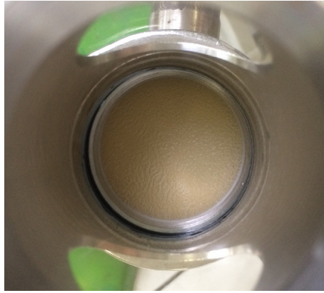
Figure 3: Photo of biofilm formed on the substrate of reactor 1
