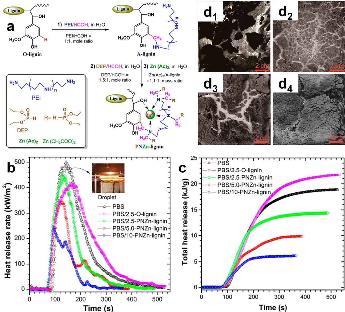
**Figure 10.** (a) Synthetic route of the functionalized lignin (PNZn-lignin); (b-c) HRR and THR curves of PBS composites at a heat flux of 35 kW/m<sup>2</sup>; and residual chars of (d<sub>1</sub>) PBS, (d<sub>2</sub>) PBS/Olignin2.5%, (d<sub>3</sub>) PBS/PNZn-lignin2.5%, (d<sub>4</sub>) PBS/PNZn-lignin10% after cone calorimeter test [119].
