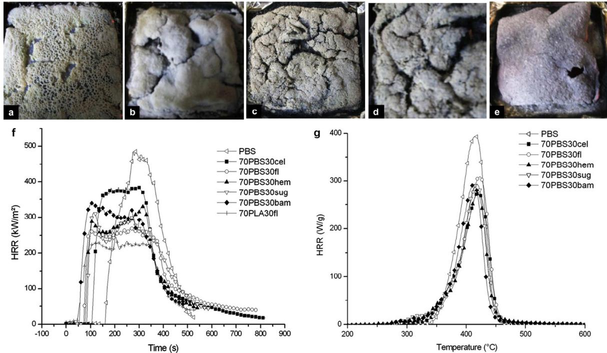
**Figure 13.** Char residues of (a) PBS/cellulose30%, (b) PBS/hemp30%, (c) 70PBS/flax30%, (d) PBS/sugar cane30%, (e) PBS/bamboo30% composites after cone calorimeter test; (f) the HRR curves of PBS/fiber composites based on cone calorimeter test at a heat flux of 35 kW/m<sup>2</sup>, and (g) HRR curves of PBS/fiber composites based on MMC test [138].
