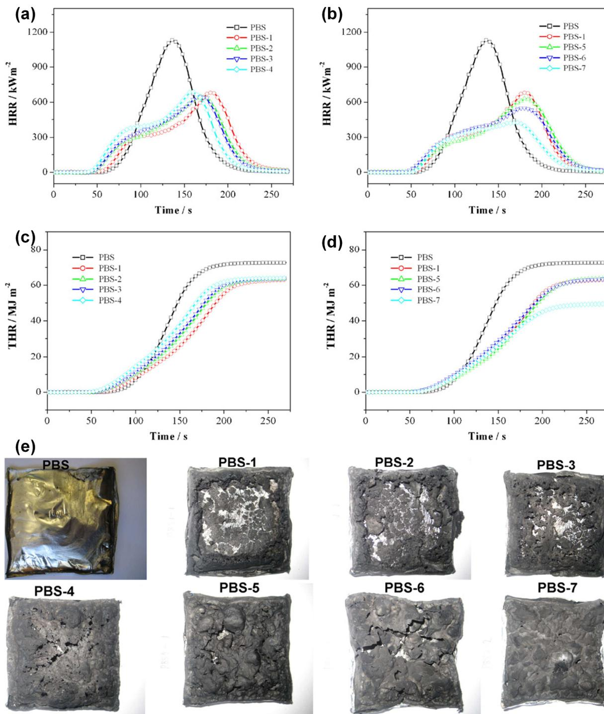
**Figure 21.** (a-d) HRR and THR curves of PBS composites at a heat flux of  $50 \text{ kW/m}^2$ ; (e) char residues after cone calorimeter test (PBS-1: PBS/MP20%, PBS-2: PBS/MP19.5%/POSS0.5%, PBS-3: PBS/MP19%/POSS1%, PBS-4: PBS/MP18%/POSS2%, PBS-5: PBS/MP19.5%/Graphene0.5%, PBS-6: PBS/MP19%/Graphene1%, PBS-7: PBS/MP18%/Graphene2%) [176].
