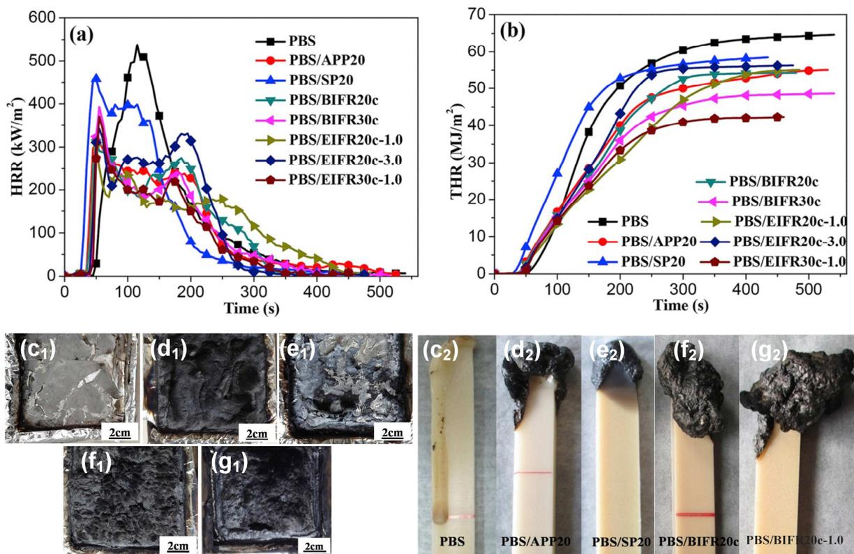
**Figure 14.** (a-b) HRR and THR curves of PBS composites at a heat flux of 35 kW/m<sup>2</sup>; residual chars of (c) PBS, (d) PBS/APP20%, (e) PBS/SP20%, (f) PBS/EIFR20%, (g) PBS/EIFR20%/HNT1% composites after cone calorimeter and LOI tests [148].
