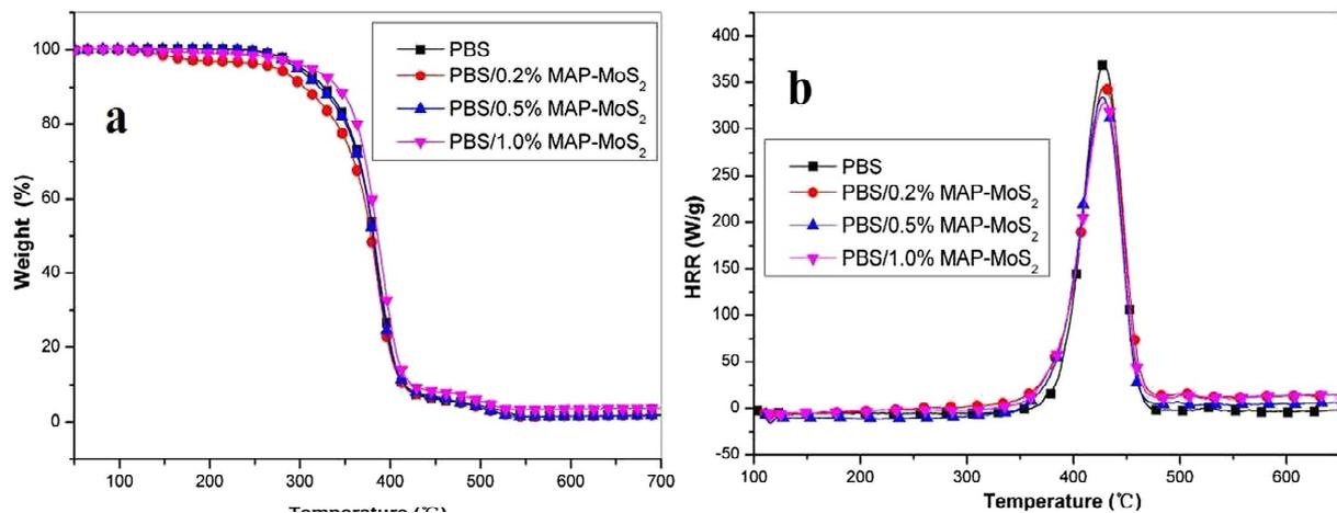
**Figure 7.** (a) TGA and (b) HRR curves of PBS composites based on TG and MCC tests [114].
