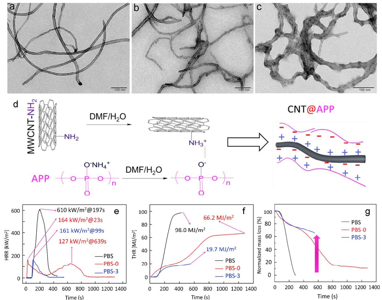
**Figure 15.** TEM images of (a) aminated multi-walled carbon nanotube (MWCNT-NH<sub>2</sub>), (b-c) CNT@APP; and (d) scheme of electrostatically APP-coated MWCNT-NH<sub>2</sub>; (e-g) HRR, THR, and mass loss curves of PBS composites at a radiant heat flux of 35 kW/m<sup>2</sup> (PBS-0: PBS/IFR20%, PBS-3: PBS/IFR19%/CNT@APP1%) [149].
