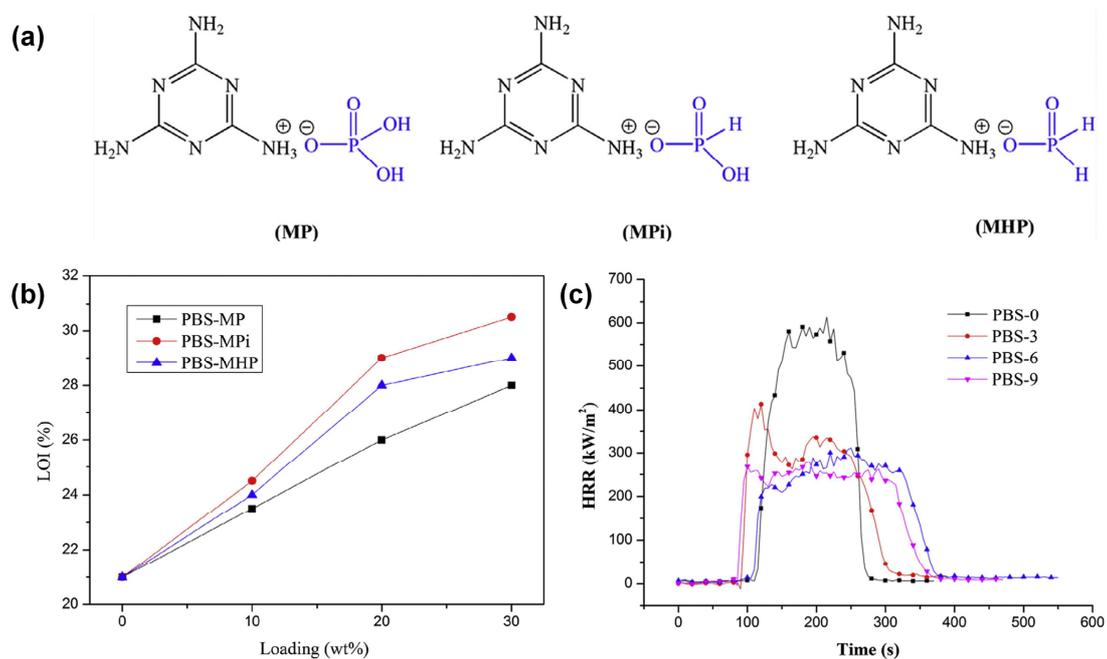
**Figure 20.** (a) The chemical structures of MP, MPi, and MHP; (b) the effect of MP, MPi, and MHP loadings on the LOI value of the PBS composites; (c) HRR curves of PBS composites at an external heat flux of  $35 \text{ kW/m}^2$  (PBS-0: neat PBS, PBS-3: PBS/MP30%, PBS-6: PBS/MPi30%, and PBS-9: PBS/MHP30%) [175].
