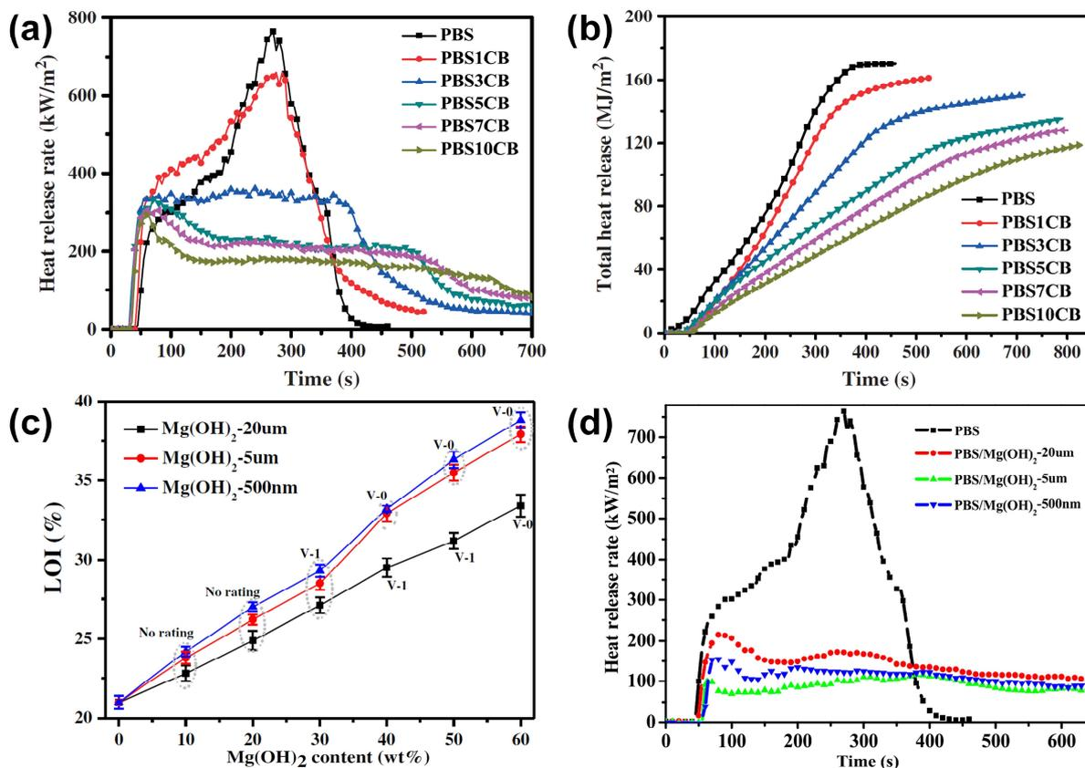
**Figure 8.** (a-b) HRR and THR curves of PBS/CB composites at a heat flux of 50 kW/m<sup>2</sup> [115]; (c) LOI, UL94 results and (d) HRR curves of PBS/MDH composites at the heat flux of 50 kW/m<sup>2</sup>[117].
