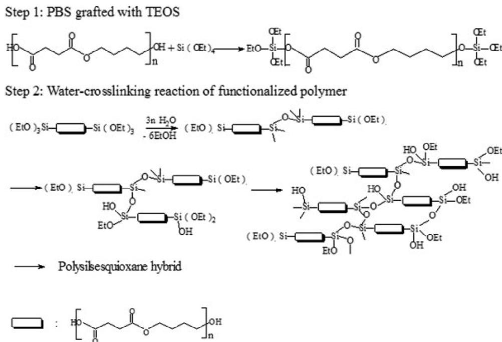
**Figure 12.** Water-crosslinking reaction mechanism of PBS/APP composites [135].
