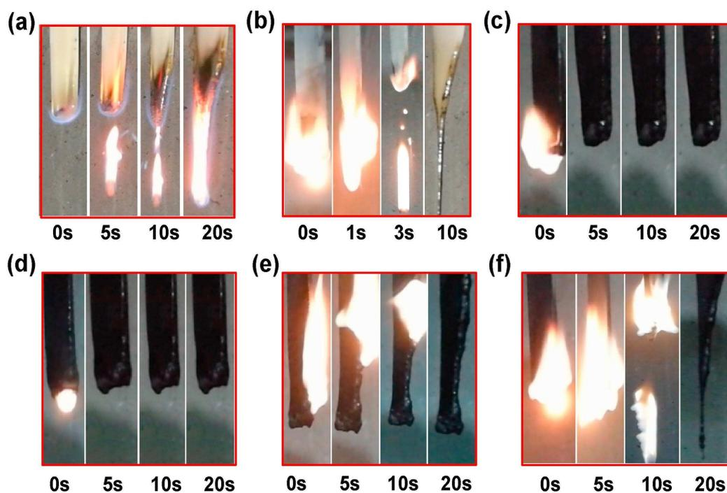
**Figure 19.** Digital photos of (a) neat PBS, (b) PBS/APP20%, (c) PBS/CAPP20% (0.1 wt.% of CNTs), (d) PBS/CAPP20% (0.2 wt.% of CNTs), (e) PBS/CAPP20% (0.4 wt.% of CNTs), and (f) PBS/APP19.8%/CNT0.2% composites during the UL-94 tests (different time after first (a) or second (b–f) ignition) [174].
