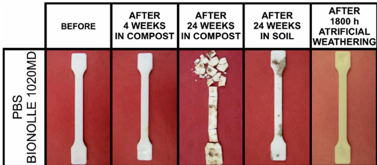
**Figure 5.** Photographs of the PBS before and after degradation [96].
