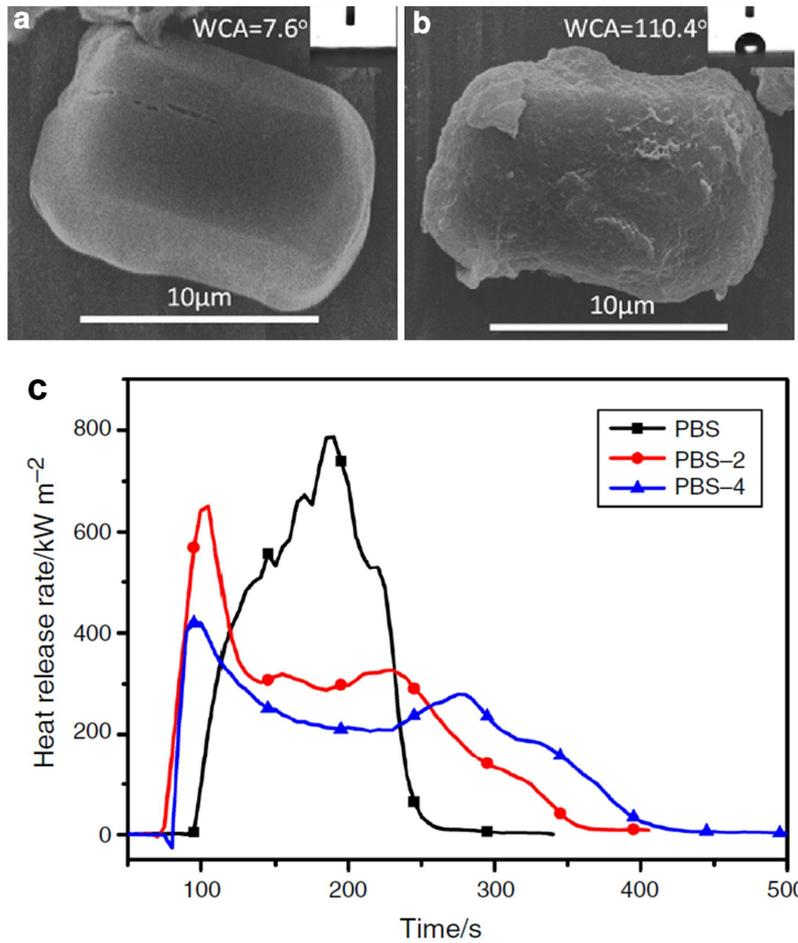
**Figure 17.** SEM images of (a) APP and (b) MAPP particles (the insets are the picture of water contact angle); and (c) HRR curves of PBS composites at a radiant heat flux of 35 kW/m<sup>2</sup> (PBS-2: PBS/APP15%/CFA5% composite, PBS-4: PBS/MAPP15%/CFA5% composite) [172].
