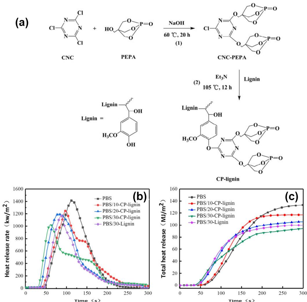
**Figure 9.** (a) synthesis route of CP-lignin; (b-c) HRR and THR curves of PBS/CP-lignin composites at a heat flux of 50 kW/m<sup>2</sup> [128].
