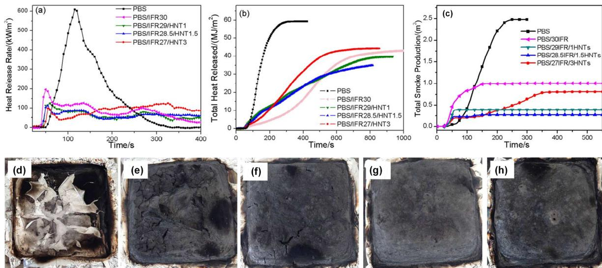
**Figure 16.** (a-c) HRR, THR, and TSP curves of PBS composites at a heat flux of 30 kW/m<sup>2</sup>; char residues of (d) PBS, (e) PBS/IFR30%, (f) PBS/IFR29%/HNT1%, (g) PBS/IFR28.5%/HNT1.5%, and (h) PBS/IFR27%/HNT3% composites after cone calorimeter test [169].
