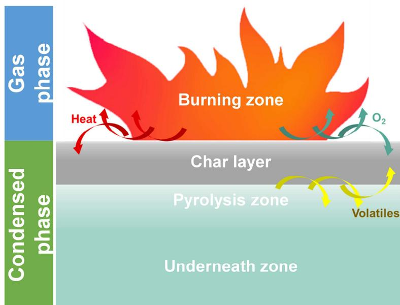
**Figure 2.** Chemical and physical behaviors of polymer combustion.
