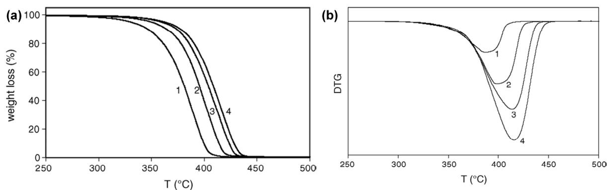
**Figure 3.** (a) TGA and (b) DTG curves of PBS at different heating rates: (1) 5 °C/min; (2) 10 °C/min; (3) 16 °C/min; (4) 22 °C/min [85].
