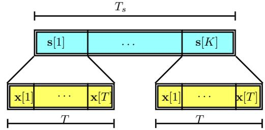
Fig. 2. Structured pilot pattern in the time domain
