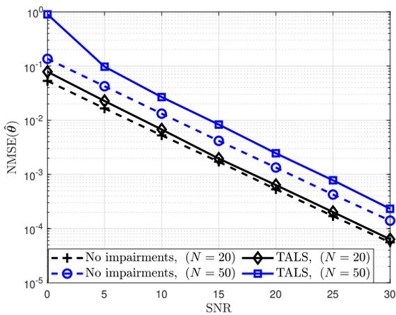
Fig. 10. TALS performance under IRS amplitude/phase perturbations.
