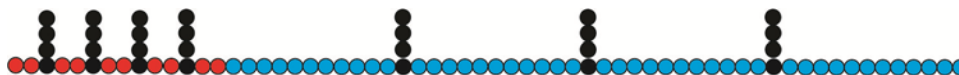
Figure 6. A typical OBC1 macromolecule with uniform distribution of short 1-octene branches (black chains) in soft blocks (red units) and hard blocks (blue units).
