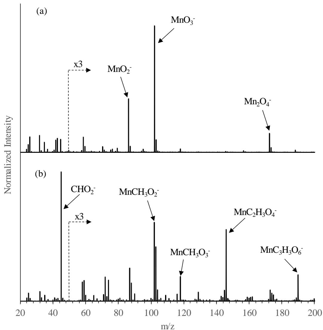
**Figure 8.** Negative ToF-SIMS spectra of (a) KB and (b) KB-F25 samples
