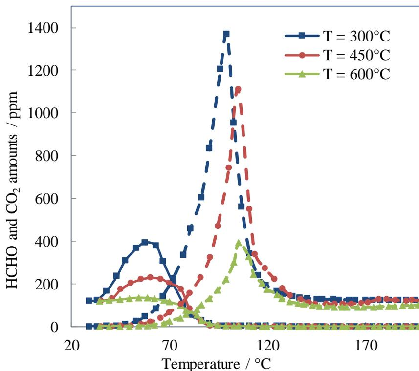
**Figure 1.** Evolution of HCHO (straight line) and CO<sub>2</sub> (dotted line) amounts in function of temperature for catalyst previously calcined at different temperatures
