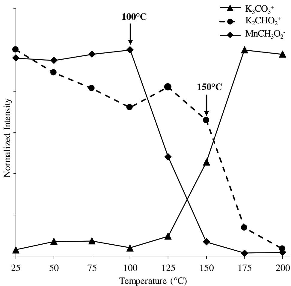
**Figure 10.** Evolution of the intensity of MnCH<sub>3</sub>O<sub>2</sub><sup>-</sup>, K<sub>2</sub>CHO<sub>2</sub><sup>+</sup> and K<sub>3</sub>CO<sub>3</sub><sup>+</sup> fragments with temperature.
