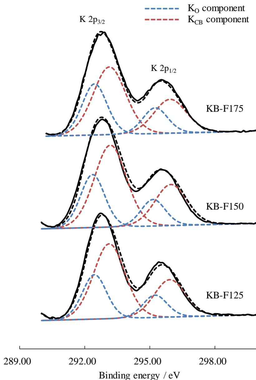
**Figure 7.** K 2p XPS signal obtained for KB-F125, KB-F150, KB-F175 samples (straight lines) and components from curve fitting (dotted lines) as a function of temperature treatment from 125°C to 175°C
