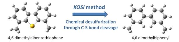
Figure 1. Desulfurization using the *KOSi* method. Using a non-catalytic process based on potassium *tert*-butoxide and hydrosilane, refractory sulfur-containing molecules found in petroleum feeds, such as 4,6 dimethyldibenzothiophene (4,6-Me<sub>2</sub>DBT) can be desulfurized. Grey, yellow, and white represent carbon, sulfur, and hydrogen atoms, respectively.
