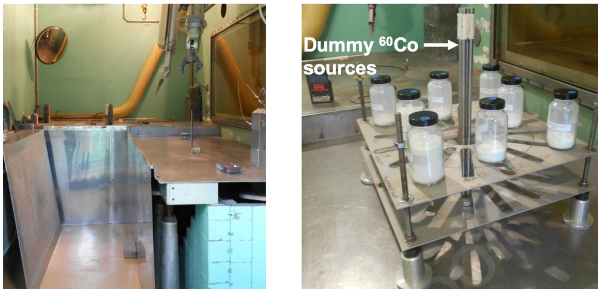
Figure 2. Interior photograph of the IRMA irradiator cell (left) and vial organization around dummy 60 Co sources (right).
