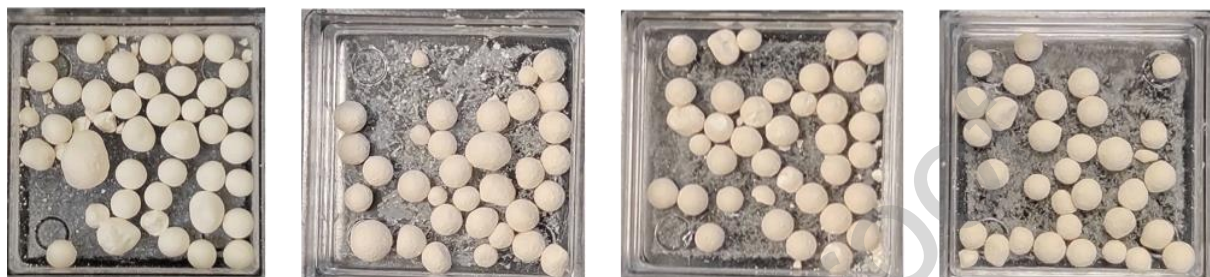
Figure 5. Photographs of binderless shaped UiO-66-NH 2 granules, with spherical size in the range 0.5-1.4 mm. From left to right: Pristine, submitted to a 2MGy dose ( \gamma radiation), submitted to water steam (120°C, 7 days), charged with 131 I then submitted to accidental conditions.
