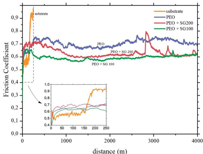
Fig. 4. Friction Coefficient for PEO specimens and substrate against sliding distance.
