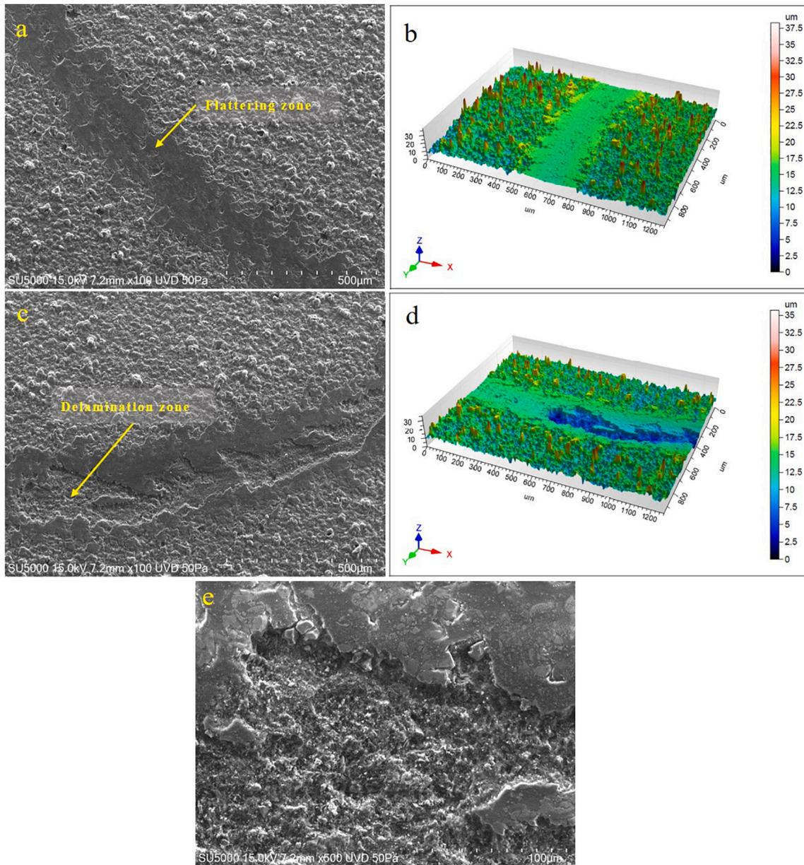
**Fig. 5.** Wear tracks obtained by SEM and wear 3D topographic surfaces obtained by confocal microscopy for PEO specimen. (a) and (b) flatter zone. (c) and (d) delamination zone. (e) magnification of the delamination zone.
