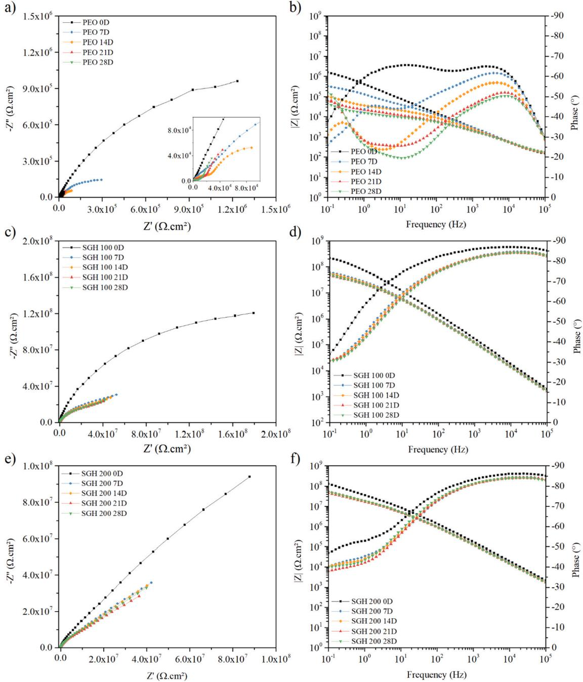
**Fig. 10.** EIS bode plots of the PEO (a, b), PEO sealed with sol-gel applied at 100 mm/min (c, d) and PEO sealed with sol-gel applied at 200 mm/min (e, f), until 28 days of immersion in 0.1 M  $\text{Na}_2\text{SO}_4$ .
