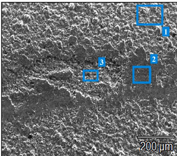
Fig. 7. SEM image of the wear track on the unsealed PEO sample and the respective EDX analysis zones.
