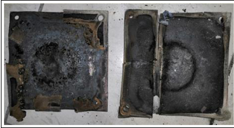
Figure 26. Sample (reference C) after testing at the bench-scale jetfire, the front face (left), and the back face showing the open junction (right).
