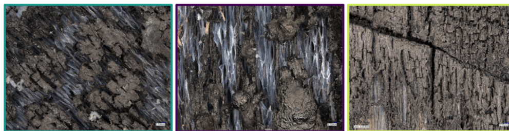
Figure 10. Observations of cone calorimeter residues: Reference (left), YB treated PEI: SPA 1:2 (center), and YB treated PEI: SPA 1:3 (right).
