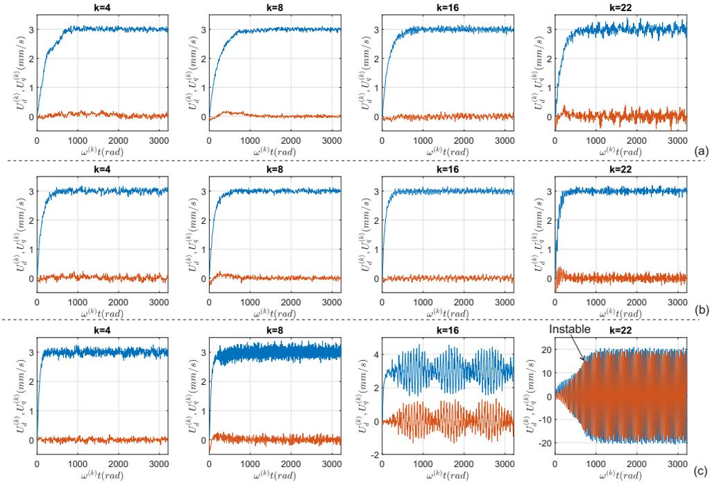
Figure 18: Closed loop time responses of the selected modes  $k = \{4, 8, 16, 22\}$ , for a simultaneous excitation,  $U_d^{(k)}$  in blue and  $U_q^{(k)}$  in red, (a)  $\alpha_k = 0.5$ , (b)  $\alpha_k = 1.0$ , (c)  $\alpha_k = 2.0$
