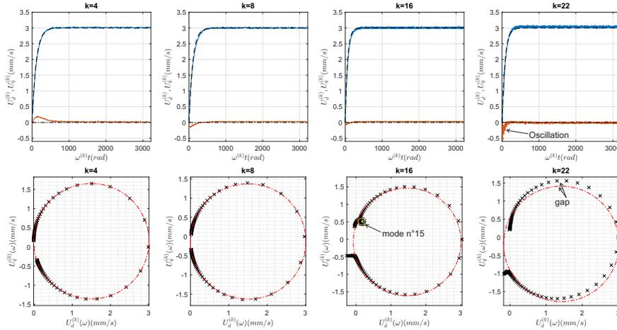
Figure 14: Time (top) and frequency (bottom) responses in the demodulated bases, with an isolated excitation. the blue and red curves in the time responses correspond respectively to  $U_d^{(k)}$  and  $U_q^{(k)}$ . The red curves in the frequency responses correspond to the identified circles
