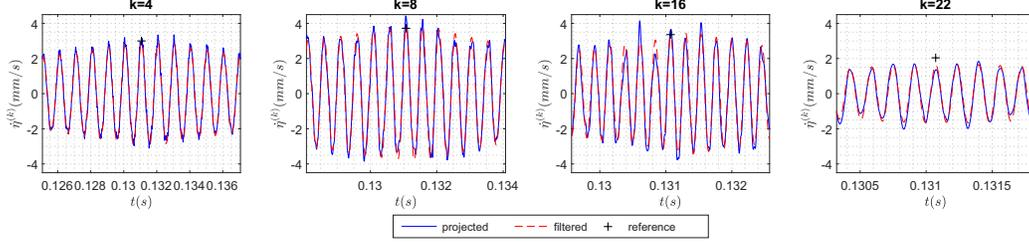
Figure 21: Extracted modal velocities  $\dot{\eta}^{(k)}$  of the controlled modes in absence of external perturbation, the modal velocities reference at the focusing time  $\dot{\eta}_f^{*(k)}$  are represented by the symbol +.
