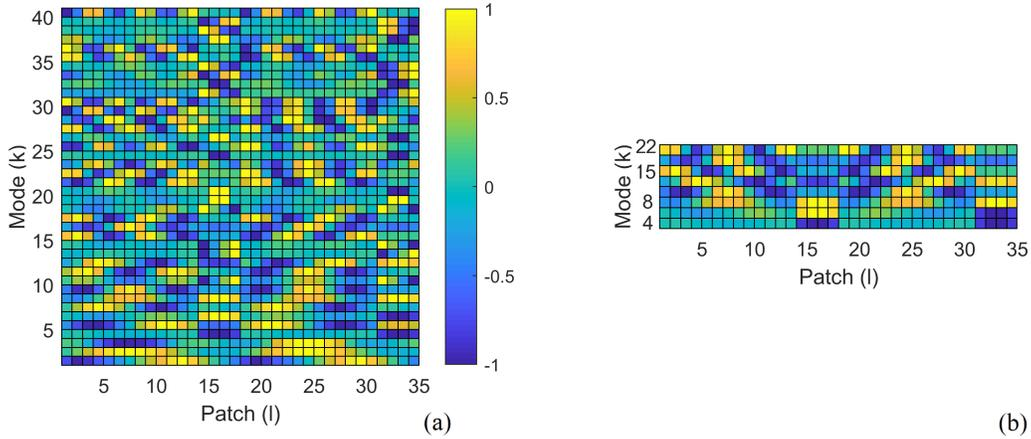
Figure 7: (a) Normalized modal coupling matrix  $\Phi$ , where each case correspond to a modal coupling gain  $\phi^{k,l}$ , (b) normalized modal coupling matrix  $\Phi(\mathbf{E})$  associated with the set of selected modes  $E = \{4, 6, 8, 9, 12, 15, 16, 22\}$ .
