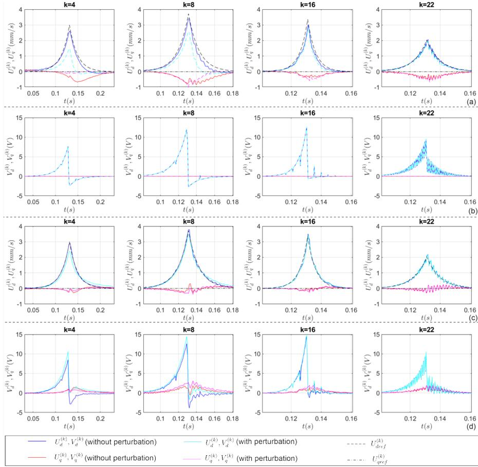
Figure 20: Modal signals in the demodulated bases for a focusing at the center of the plate, with  $t_f = 131.1\text{ms}$ : (a) Modal velocities components  $U_d^{(k)}$  and  $U_q^{(k)}$  in the case of just feedforward control  $\mathbf{C}_{\text{FF}}$ ; (b) The associated voltages  $V_d^{(k)}$  and  $V_q^{(k)}$
