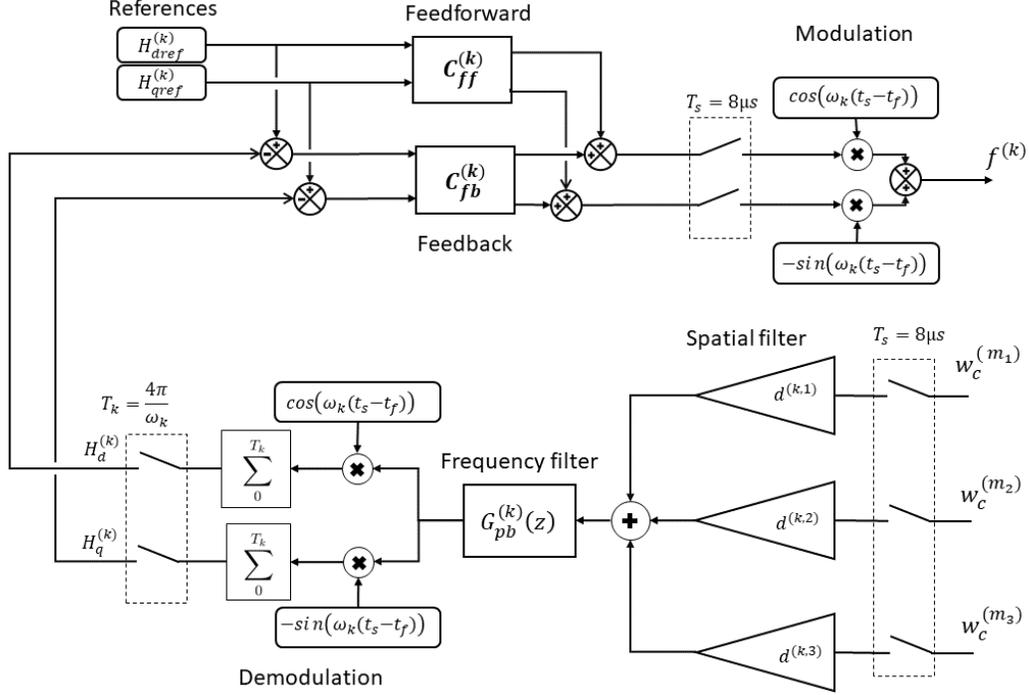
Figure 19: Control structure for one vibration mode
