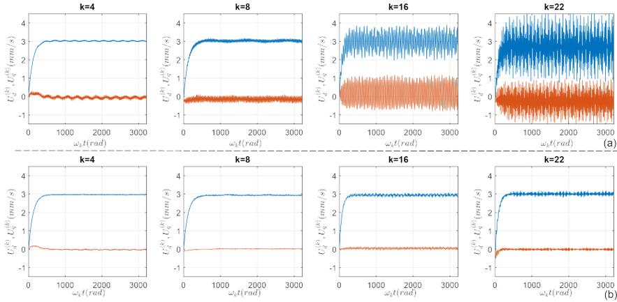
Figure 17: Influence of the modal filter on the measurement of the modal velocities,  $U_d^{(k)}$  in blue and  $U_q^{(k)}$  in red : (a) measurement responses by using only the demodulation bloc with an arbitrary sensor ; (b) measurement modal velocities while applying the proposed spatial frequency filter
