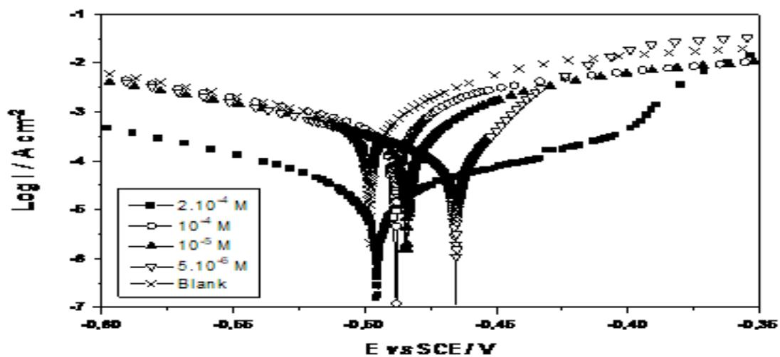
Figure 2.a. Polarization curves for C38/1M HCl system containing different concentrations of TO1.
