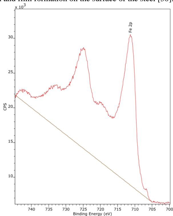
**Figure 7.** XPS spectra of Fe2p<sub>3/2</sub> and Fe 2p<sub>1/2</sub> for C38 steel treated by **TO1** in HCl 1M.
