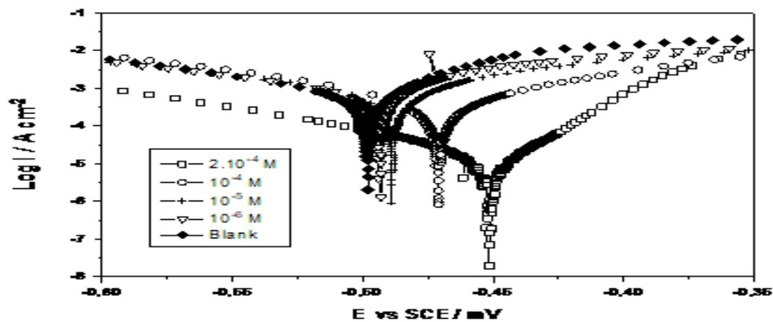
Figure 2.b. Polarization curves for C38/1M HCl system containing different concentrations of TO4.
