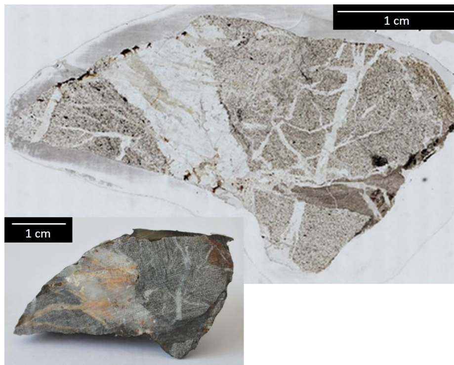
Figure 2 : Main petrographic features of the studied sample. General view of the shale sample and of the thin section, on which the veins can be seen in white through the shale in grey (natural light).
